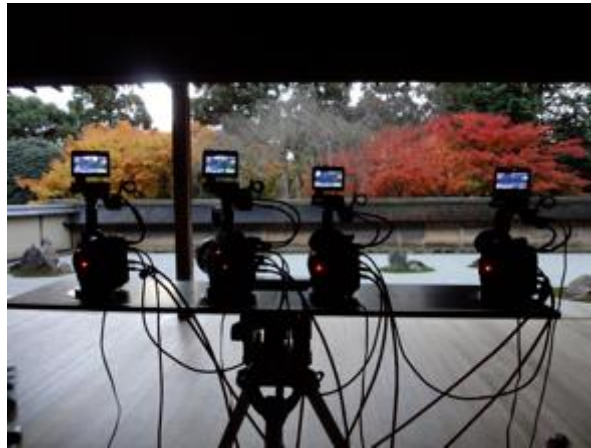
FIGURE 13 Camera array consisting of four 4K cameras
