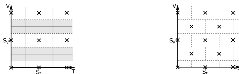
(c) A pure vertical filter in the progressive sampling structure. shaded areas are the filter stop-band. reduces vertical detail equally for slow- and fast-moving areas
