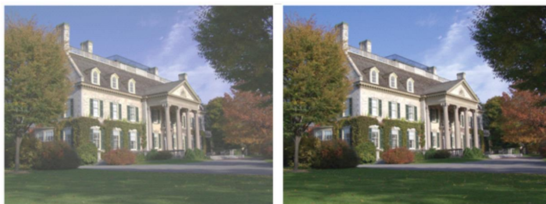
FIGURE 8 The left image has a system transfer function (or greyscale) of unity slope. The right image has a system transfer function consistent with ITU broadcast practices
