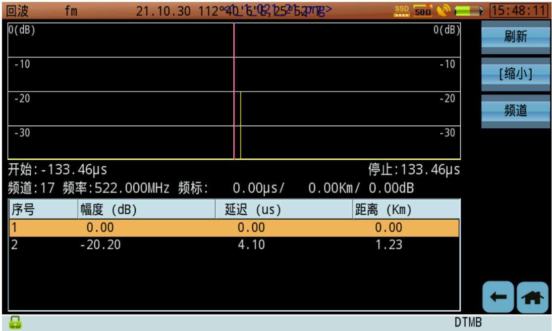
Multipath parameters of test site No. 1 before optimization
