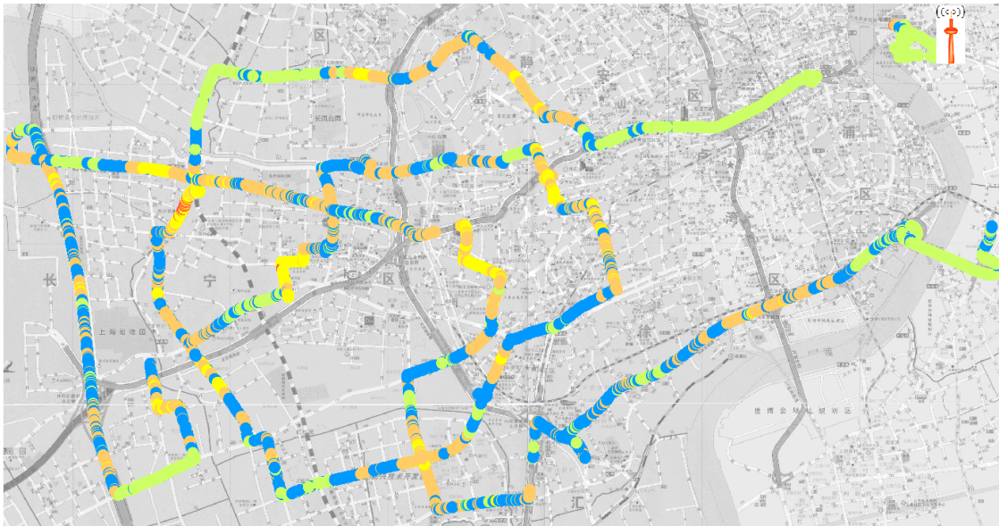
FIGURE P4-4 DTMB Coverage map – only with the broadcasting of Oriental Pearl station
