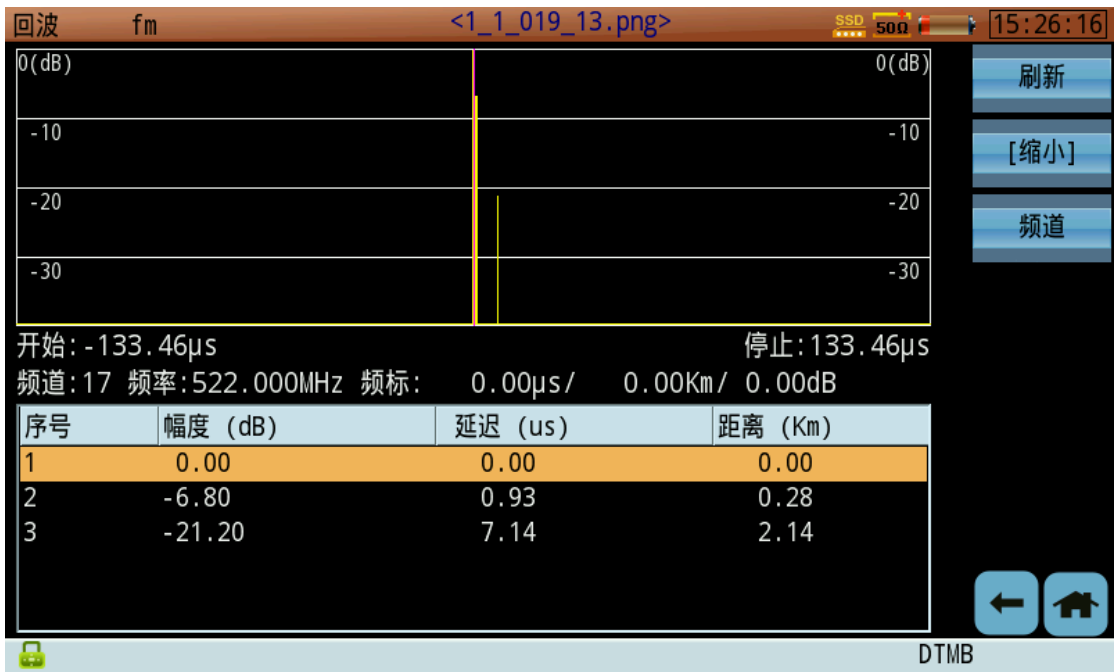
Multipath parameters of test site No. 2 before optimization
