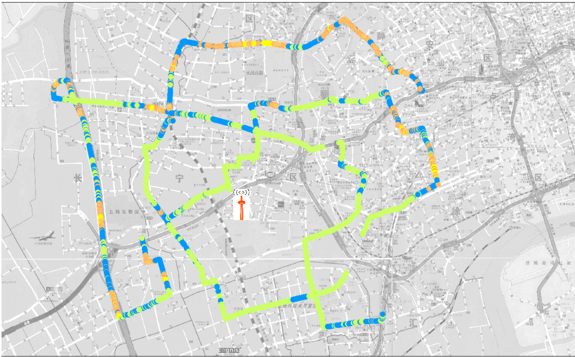
FIGURE P4-5 DTMB Coverage Map – only with the broadcasting of HongQiao station
