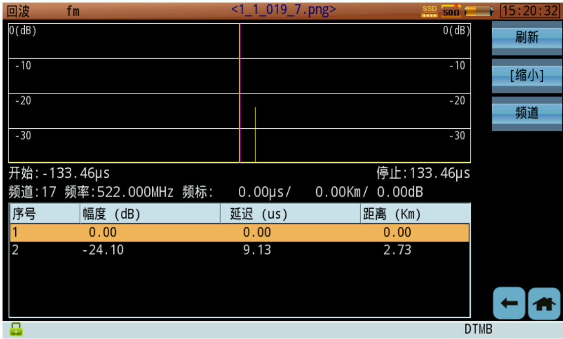
FIGURE P4-51 Multipath parameters of test site No. 2 after optimization
