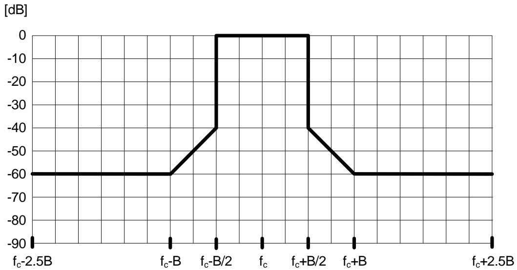
FIGURE 37 Transmit spectral power mask for WMAS, RBW = 100 kHz, Peak Detector
