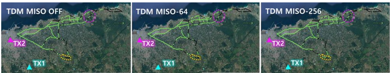
(d) Reception success (green mark) and failure (black mark) for the TDM configuration
