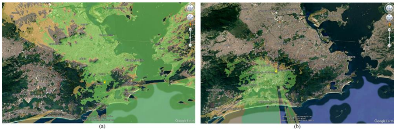
FIGURE 108 DTV+ Pilot Stations field strength predictions
