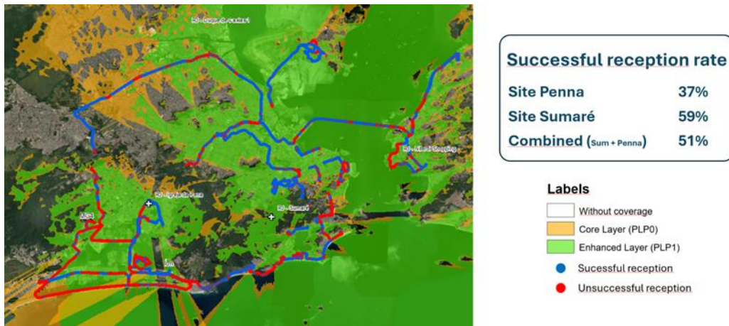
FIGURE 111 Antenna design 3 and Receiver 3 – Reception success rate
