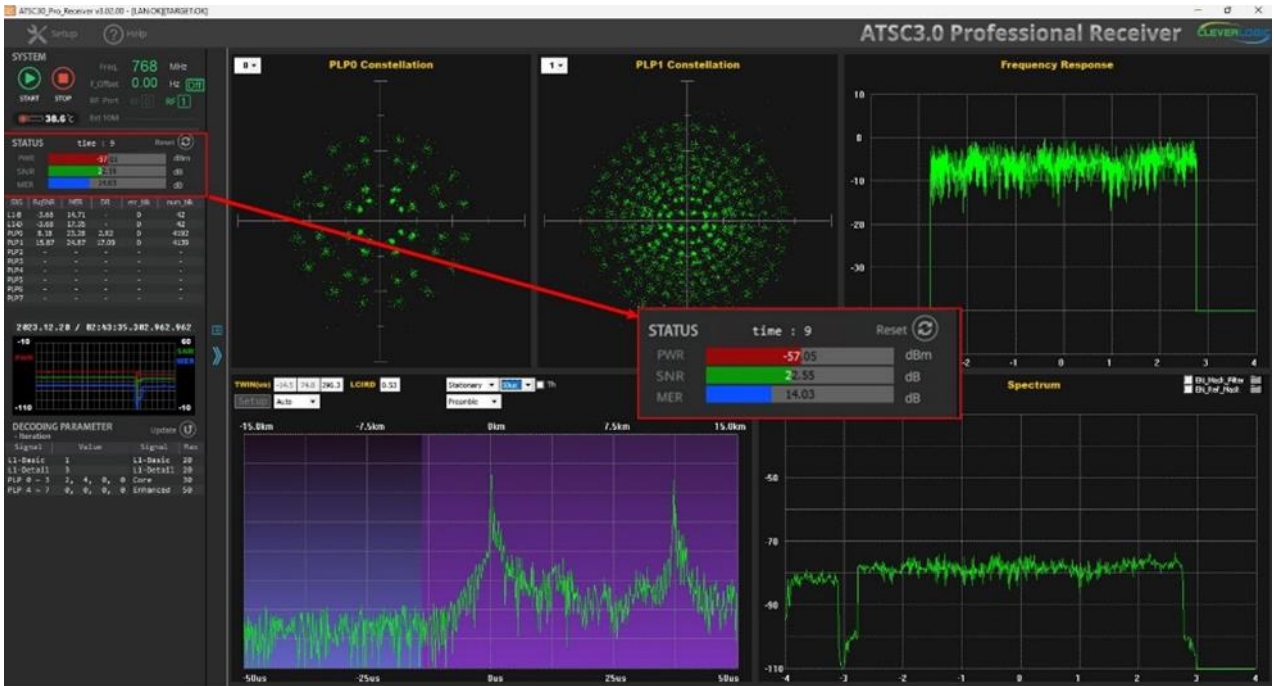
Signal characteristics of input to Integrated-MATV system (measured at antenna stage)
