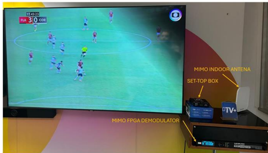
FIGURE 106 DTV+ indoor reception setup
