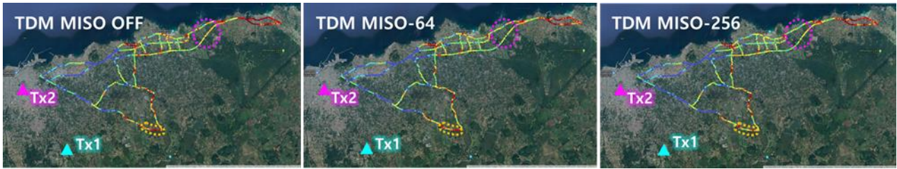
(c) Reception success (green mark) and failure (black mark) for the LDM configuration
