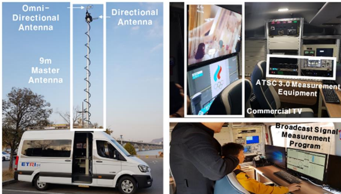
FIGURE 45 ATSC 3.0 field test configuration – Field measurement facilities
