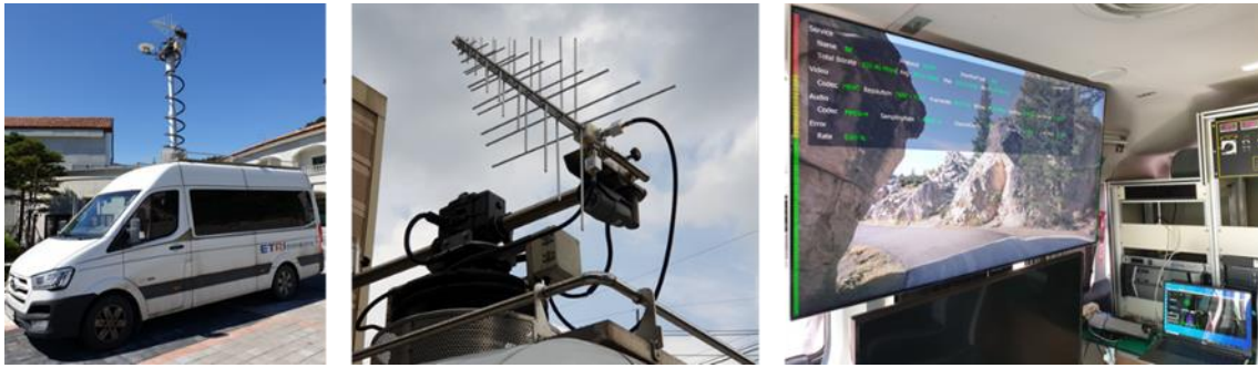
FIGURE 63 ATSC 3.0 MIMO measurement test vehicle
