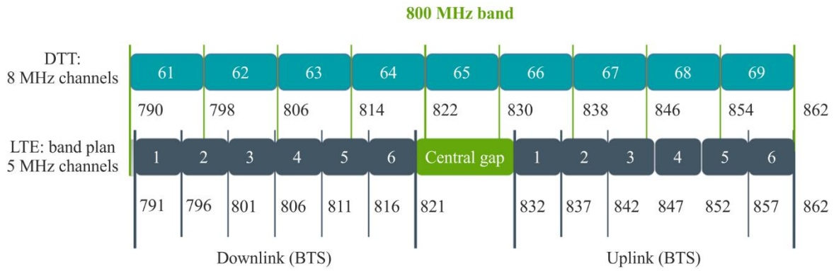
FIGURE A4.1 Overlap between DTTB channels 67, 68 and 69 and 800 MHz LTE
