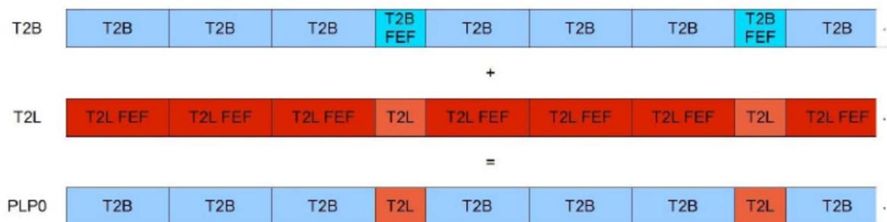
For the second case the increase of the FEF block length in T2-Lite is employed in order to accommodate the long T2-Base blocks.
