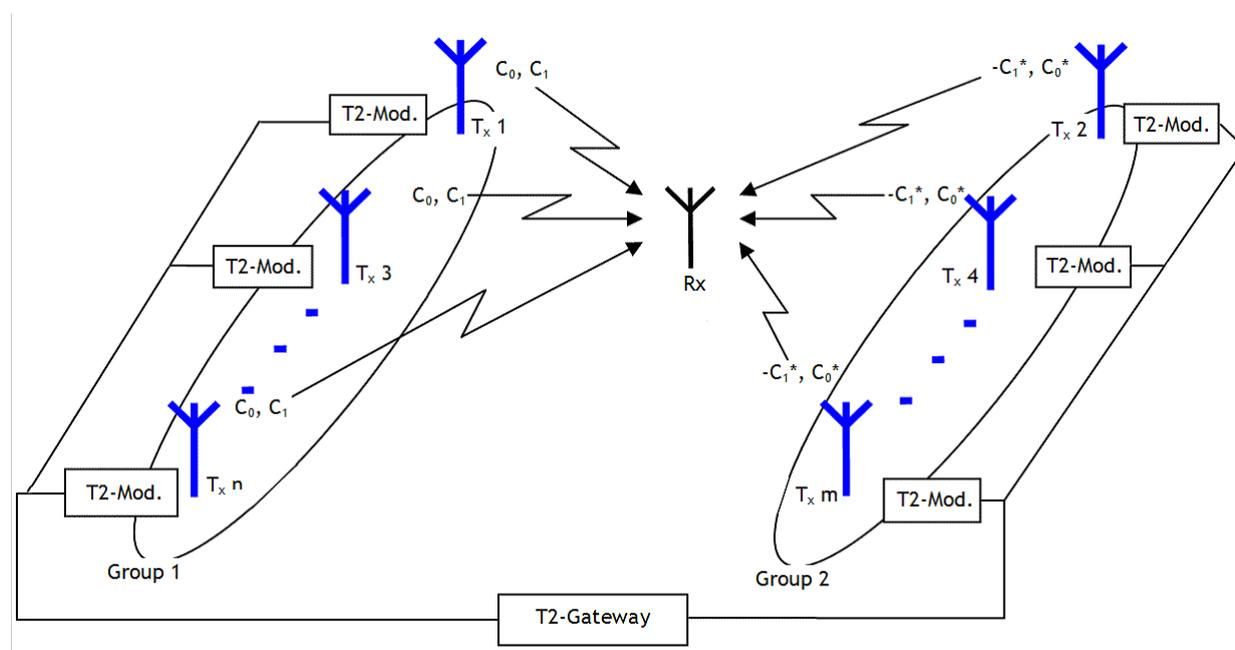
A DVB-T2 MISO network should be viewed as a particular form of an SFN, as the multiple transmissions require synchronization and timing in much the same way as a ‘standard’ SFN.
