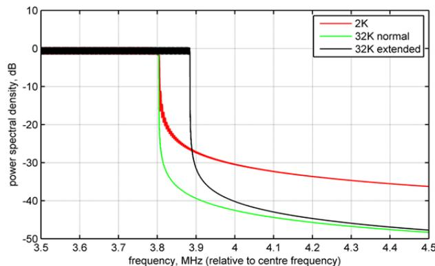
Because of its higher number of usable carriers the extended carrier mode has an increased data capacity as the normal carrier mode. Table 2.20 gives the gain of the extended carrier mode for the different FFT modes.
