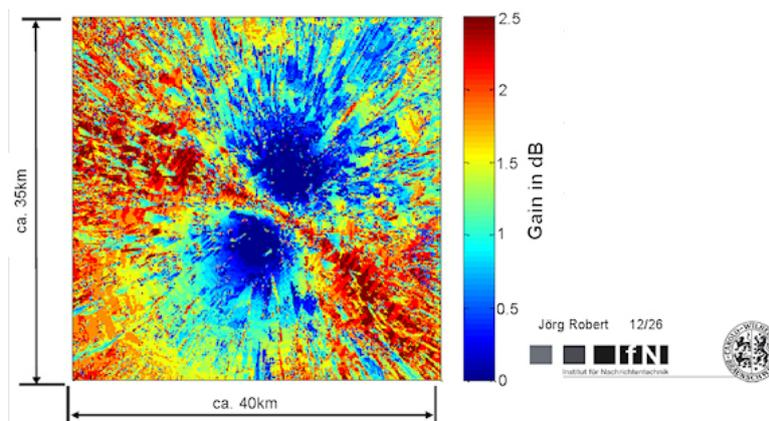
Additional gain is achieved outside the core coverage areas of the two transmitters. With regard to acceptable indoor reception the coverage gain amounts to 30% in this simulation.
