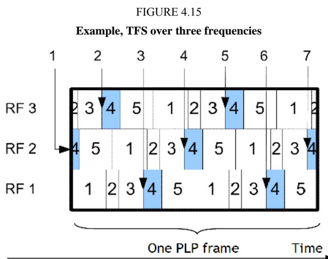
In Fig. 4.15 each physical layer pipe (PLP) is spread out over all (here 3) RF channels and over time. Each PLP is interleaved within the physical layer (PL) frame resulting in much improved time and frequency diversity.
