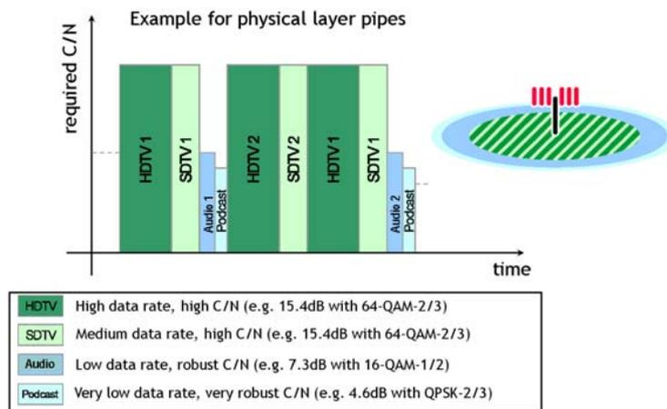
An example is given in Fig. 4.20 where four different classes of services (HDTV, SDTV, Audio Broadcasting and Data Broadcasting) are carried in one multiplex. Each of the services has a different data rate and a different coverage radius indicated in the Figure on the right hand side.
