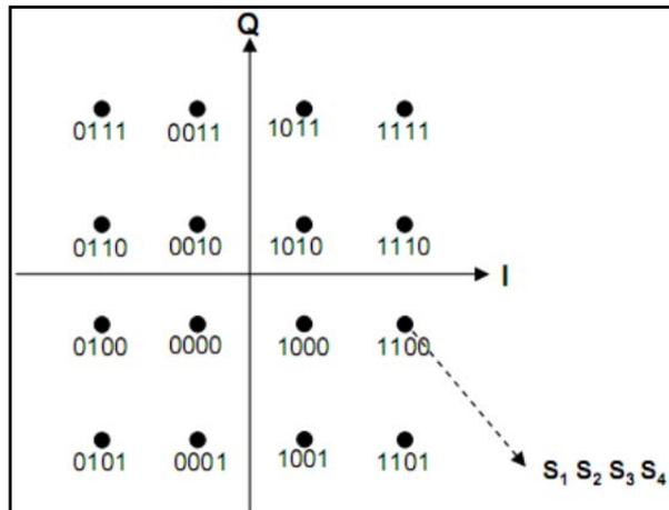
There are various ways of attributing the bits to the symbols. Best results are achieved if only one bit is changed when going from one symbol to the next closest symbol. In this way only one bit is mistaken when a symbol mismatch occurs with the next closest symbol. This coding is called Gray mapping. Figure 2.3 shows a Gray mapping constellation.
