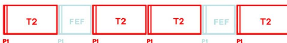
FEFs can be used for Transmitter Signatures [A150]. They allow measurements to identify which echo (path) in the channel impulse response originates from which transmitter of the SFN. It is also possible to display the parts of the channel impulse response originating from individual transmitters of the SFN.
