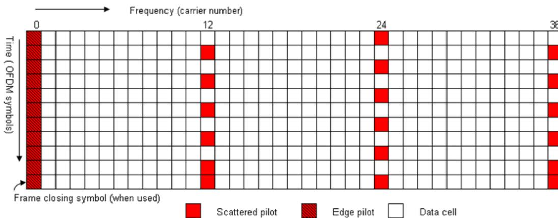
Table 60 of [EN 302 755] shows that the carrier spacing for a DVB-T2 32k mode is 279 Hz. A scattered pilot spacing of 1 in 12 therefore means that pilots occur every 3.348 kHz. At this point, it should be noted that the Nyquist rate of real valued signals (i.e. signals with no imaginary component) is equal to twice the maximum frequency within the signal, which is widely
