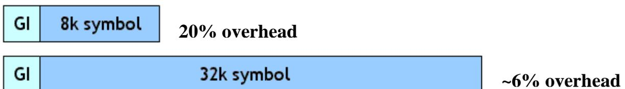
For mobile reception in UHF Band IV/V, or higher bands, smaller FFT sizes should be used as they offer better Doppler performance. The 1k FFT mode which offers the highest Doppler performance is intended primarily for operation in the L-band (about 1.5 GHz), or higher, using a nominal occupied bandwidth of 1.7 MHz. Given that the fundamental sampling rate is lower, the carrier spacing will be correspondingly smaller than it would be in an 8 MHz channel.
