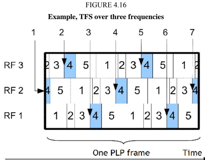
In Fig. 4.16 each physical layer pipe (PLP) is spread out over all (here 3) RF channels and over time. Each PLP is interleaved within the physical layer (PL) frame resulting in much improved time and frequency diversity.
