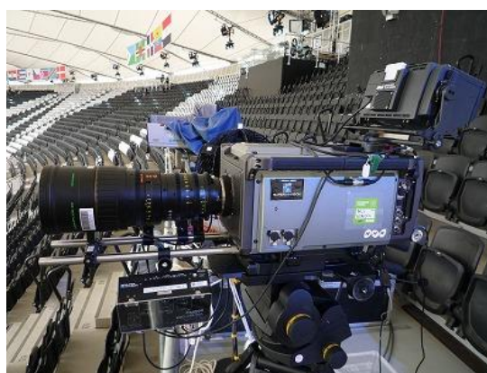
FIGURE 54 1.25-inch 4-CMOS camera and 5x lens
