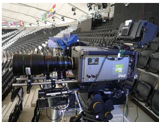
FIGURE 54 1.25-inch 4-CMOS camera and 5x lens
