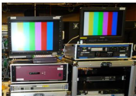
8K-4K down-converter and 28-inch 4K screen for monitoring (left)
