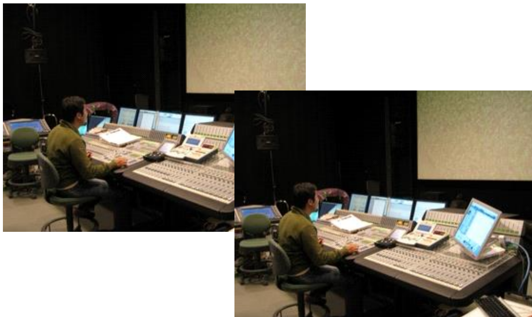
FIGURE 25 22.2 multichannel sound mixing console
