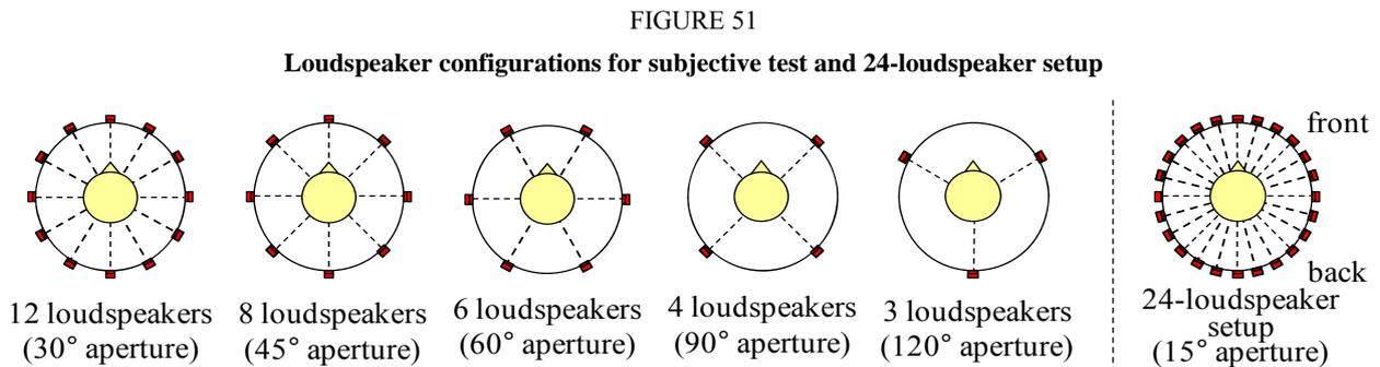
The stimuli comprised white noise with 1 s duration and 50 ms rise and fall time. The stimuli were reproduced by two adjacent loudspeakers with amplitude difference for each loudspeaker configuration. The pair-wise amplitude panning method of tangent law was used to derive the gains of the two adjacent loudspeakers. This law is shown in equation (1).
