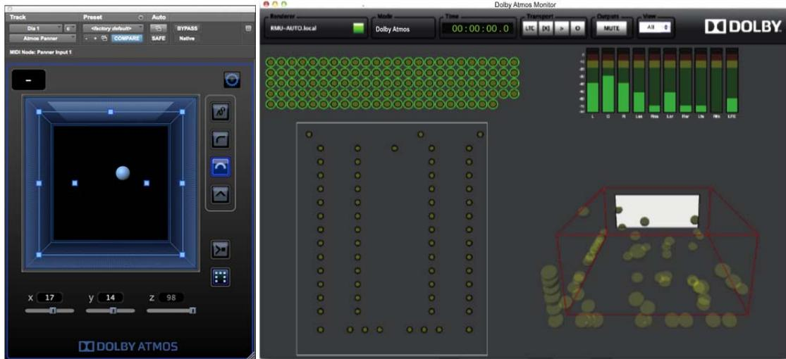
During authoring, the state of the entire mix can be monitored using a separate application (Fig. 32b). This representation shows object activity status and input levels and 9.1 output metering information. The representation also includes a 3D spatial display of the room and object positions, as well as a speaker view showing current loudspeaker configuration and output levels.
