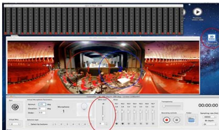
The outputs of the virtual microphones can be fed directly from the operator's computer to an audio mixer or to a recording system.
