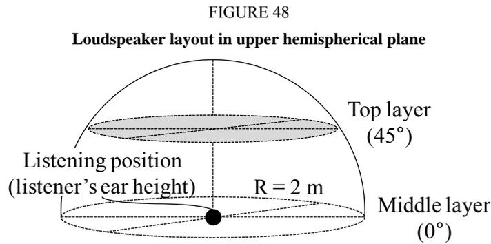
We evaluated nine test conditions for loudspeaker configurations, five using a single (middle) layer and four using both the middle and top layers. These conditions are shown in detail in Fig. 49.
