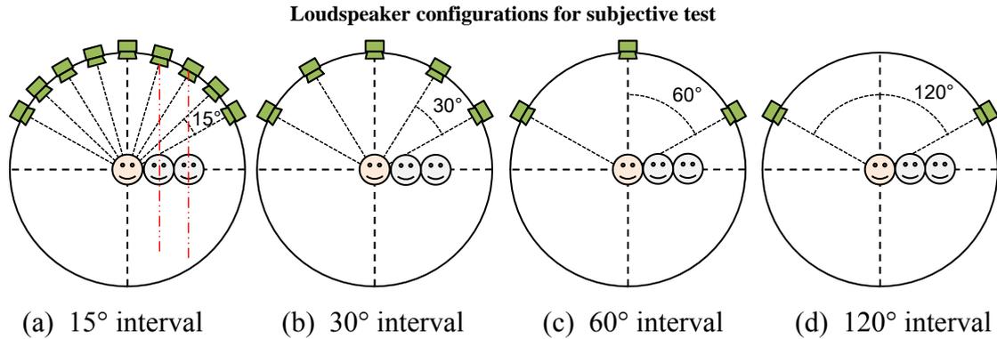
We used certain portions of the nine loudspeakers to evaluate four test conditions for loudspeaker configurations. These conditions are shown in detail in Fig. 57. For each loudspeaker configuration seventeen desired azimuth angle conditions of the sound images were set from  $-60^\circ$  (left) to  $60^\circ$  (right) with  $7.5^\circ$  intervals by two adjacent loudspeakers.
