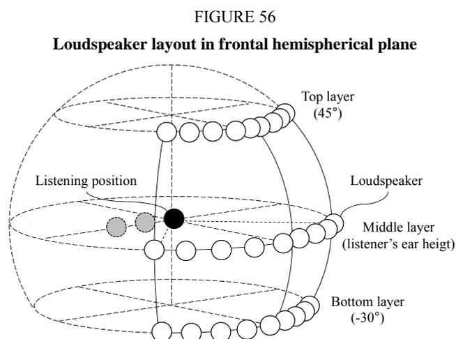
Nine loudspeakers were placed at a 15° interval for each layer as shown in Fig. 57(a). The distance between a listener and each loudspeaker was 2 m. To exclude the visual influence on loudspeakers, an acoustically transparent but visually opaque curtain was installed between the loudspeakers and a listener. Labels were set to indicate the azimuth angle at each 1° interval to respond the perceived azimuth angle.
