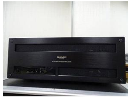
FIGURE 10 ISDB-S3 receiver for 8K UHDTV
