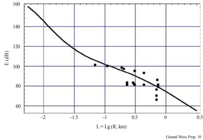
From the figure it may be seen that the measured data satisfactorily agree with the calculated curve. It is important to note that the experimental data are clustered together, not dropping out even when the measurements were carried out inside buildings. Exceptions occurred for measurements carried out in a lift, where the additional attenuation by metal walls was up to 40 dB.
