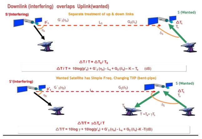
$\eta_S$  = Direction, from Interfering Satellite S', of Wanted Satellite S
