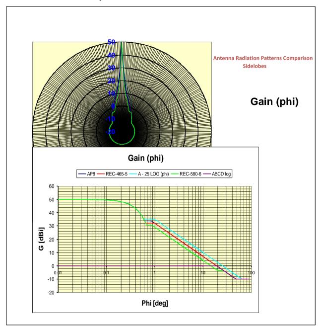
The following diagram shows how the mainlobe is modified when the antenna diameter is changed, observing a reduction of interference of approximately 5 dB to a satellite located at 1 degree of separation while increasing the antenna diameter from 1.2 to 13 metres.
