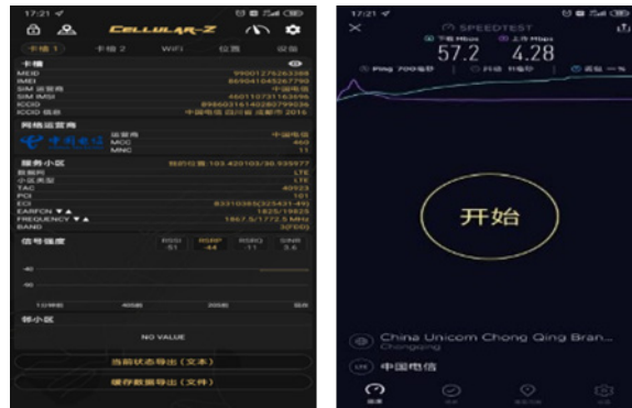
Figure 9A: Screenshot of service testing data of the 4G backpack base station
