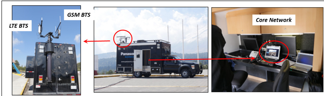
Figure 11A: Local Cellular System (LTE and GSM)
