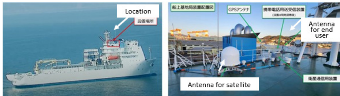
Figure A-38: Shipboard base station
