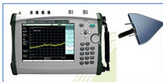
Figure A-30: Spectrum analyser with directive antenna
