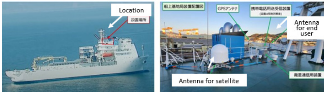
Figure A-38: Shipboard base station
