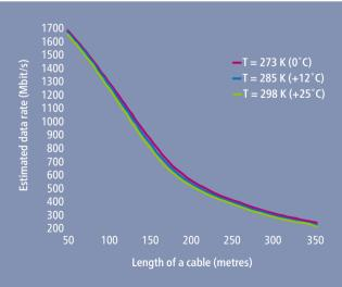
Figure 4 — Data rate decrements of 212 MHz G.fast towards the reference temperature of 0°C
