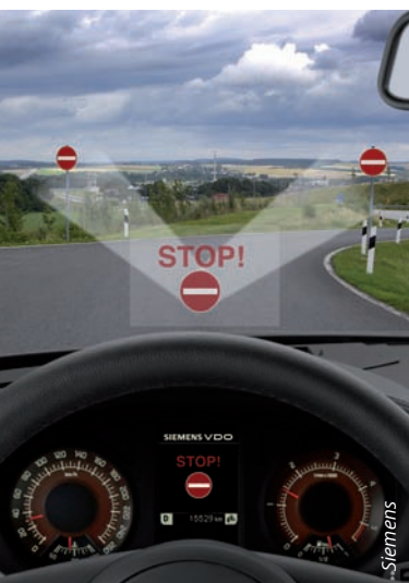
Warning of potential wrong-way driving
