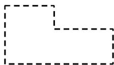
An <option symbol> logically contains the whole of any one-dimensional graphical symbol cut by its boundary (that is, with one end point inside).
