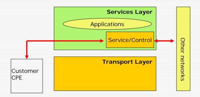
A key service is VoIP and the service/control module manages the QoS on connecting IP to circuit-switched calls
