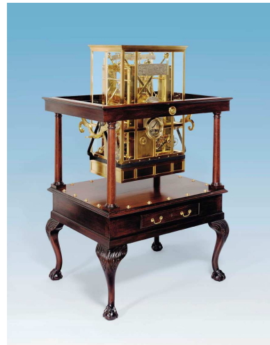
Working model of Harrison's second marine timekeeper
