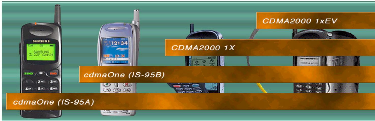
cdmaOne™ identifies 2G and 2.5G cellular, PCS and wireless local loop (WLL) services based on the IS-95A and IS-95B CDMA air interface standards. IS-95A supports data delivery up to 14.4 kbps while IS-95B offers up to 115 kbps.
