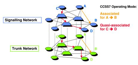
The path used by the Signalling Messages may be different from the path in the trunk network, because signalling and trunk network are logically independent!
