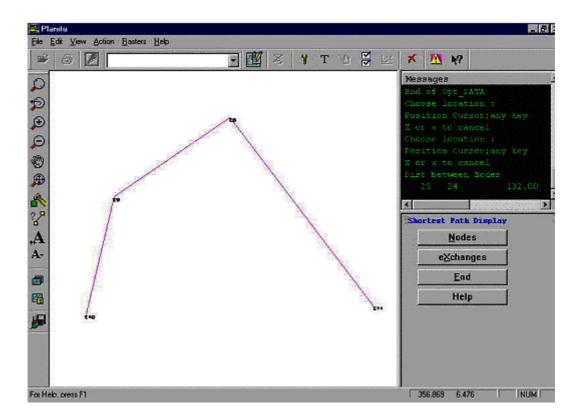
Some times is difficult to read node names, as access nodes and transport nodes are in the same location (program will ask confirmation by prompting the nod name).
