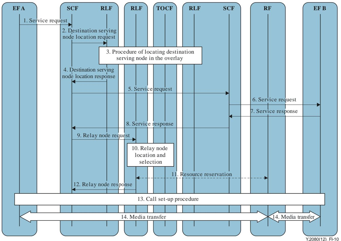
**Figure I.10 – Providing MMTel service with a relay node**
