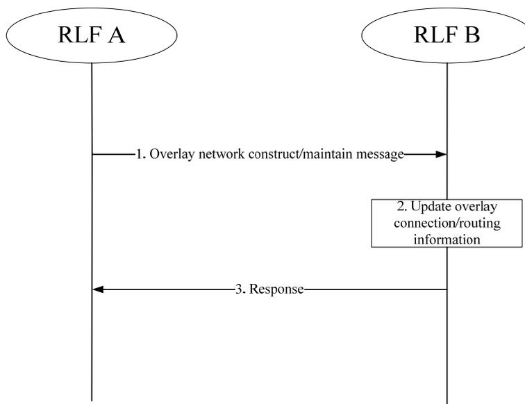
**Figure 7-3 – Exchanging information to construct and maintain the overlay**
