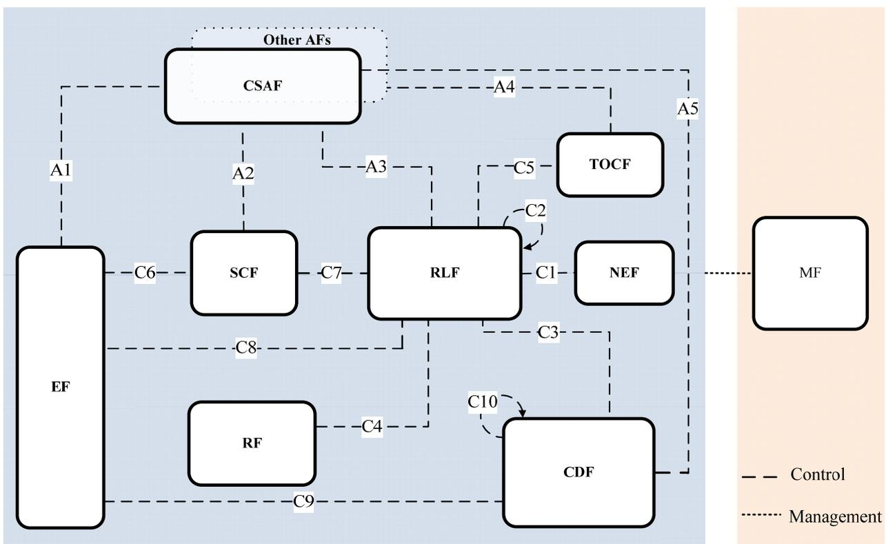
NOTE – This figure shows the interfaces for the control plane only. Media data transmission and transmission control are conducted through media interfaces depicted in Figure A.1.
