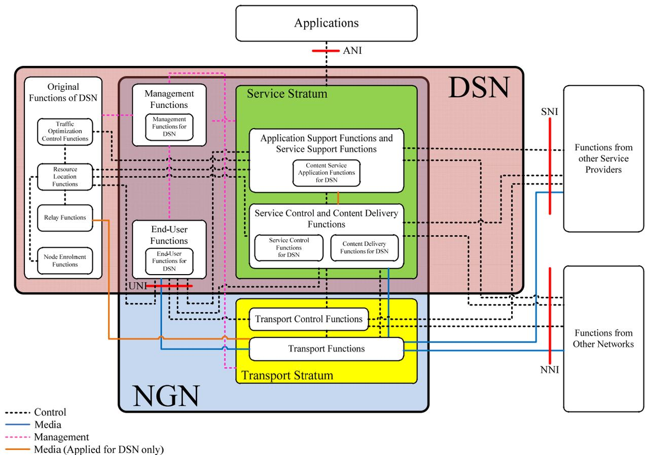
**Figure A.1 – Relationship between the DSN and NGN from a functional architecture view**
