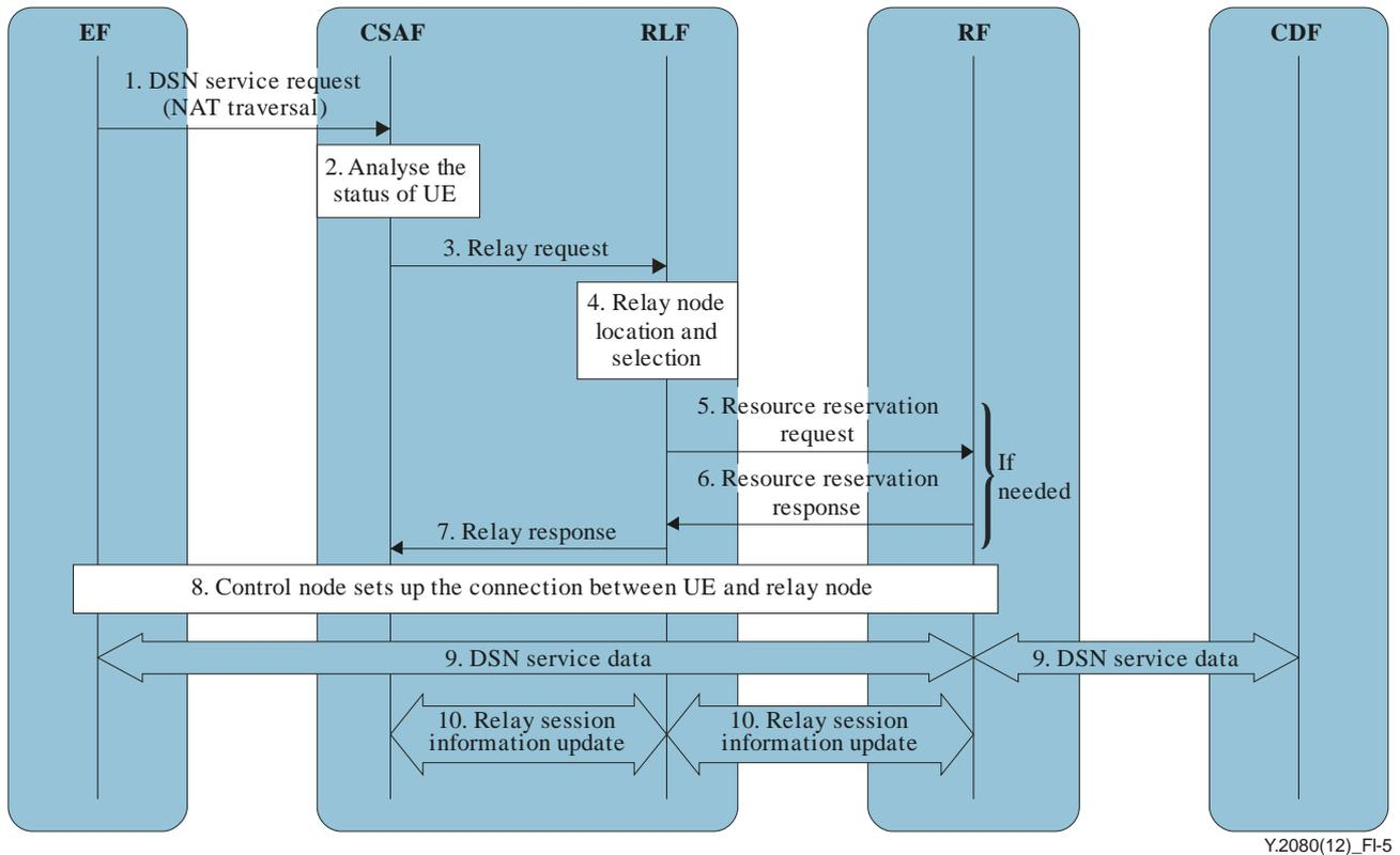
**Figure I.5 – Providing DSN services through the relay node (NAT traversal based on the RF)**
