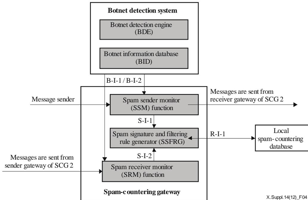
**Figure 4 – Working procedure of the reference model**
