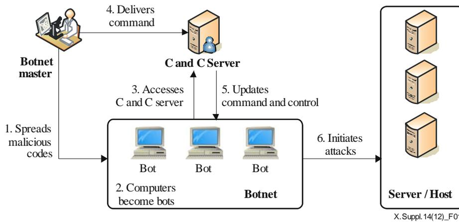
**Figure 1 – Common working procedure of a botnet**
