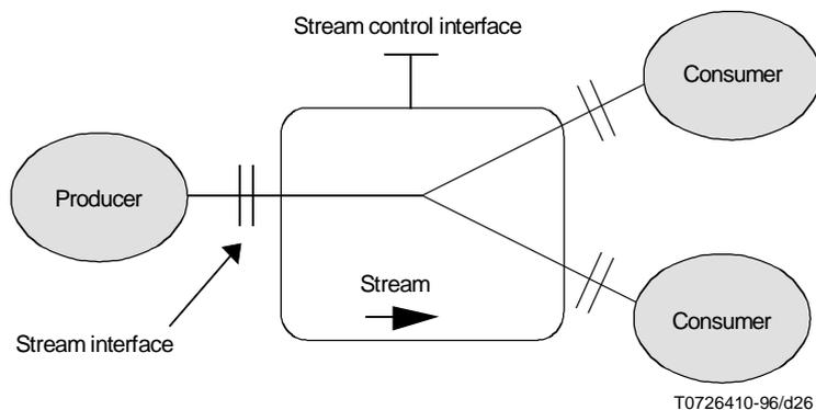
Figure 26 – Representation of an explicit binding (e.g. stream)
