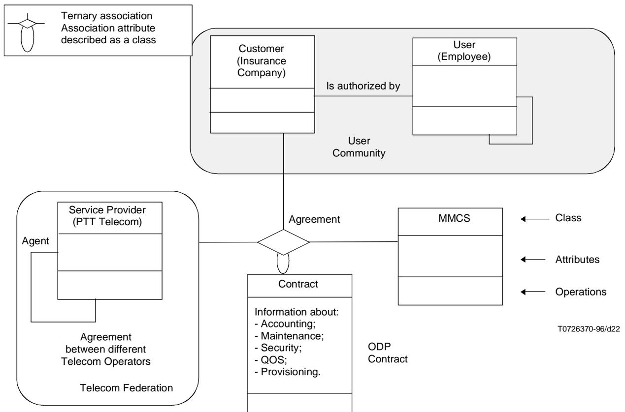
Figure 22 – ODP Enterprise specification using OMT graphical notation
