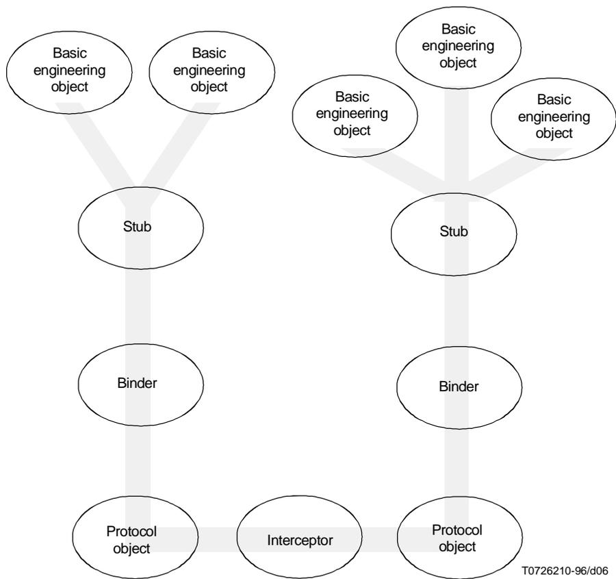
Figure 6 – An example of a group channel configuration
