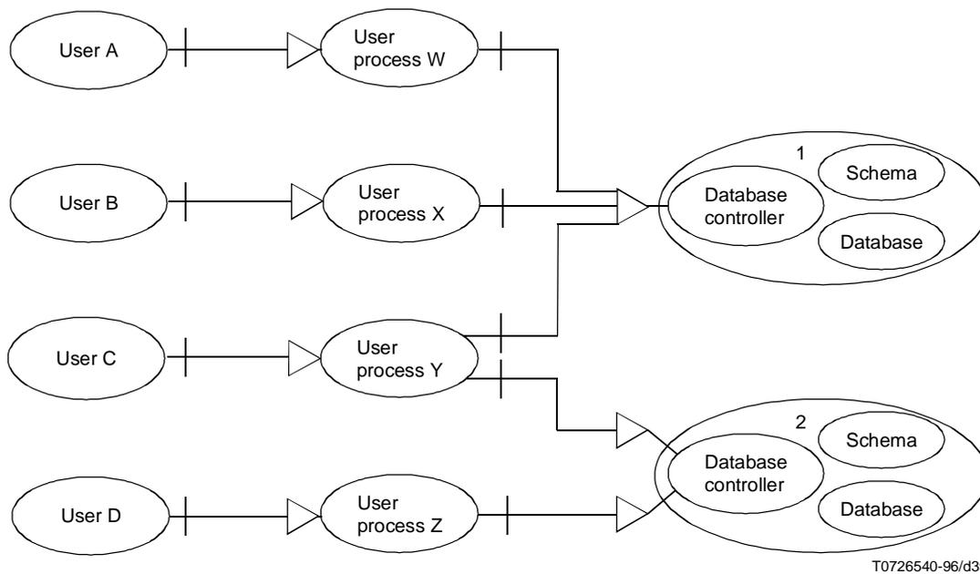
**Figure 39 – Order processing system – Computational specification**
