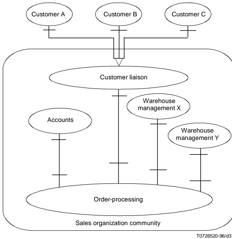
**Figure 37 – Order processing system – Enterprise specification**
