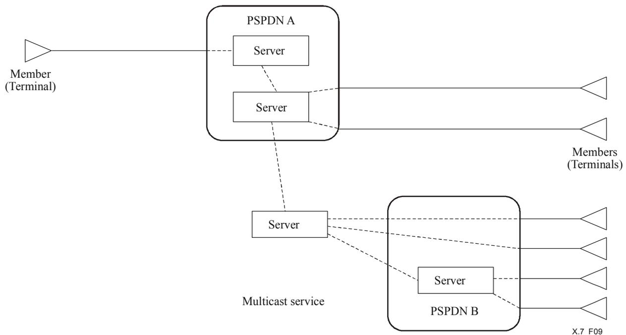
**Figure 9/X.7 – Example of multicast server implementation**
