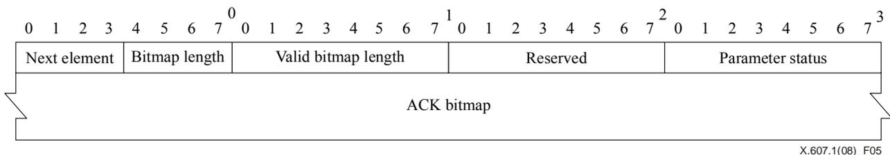
**Figure 5 – Acknowledgment extension element**
