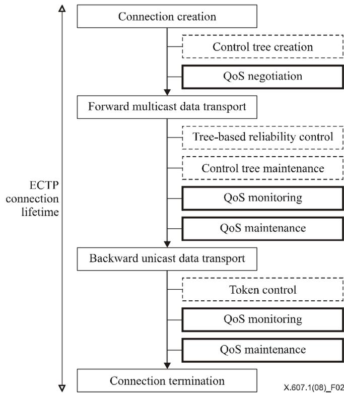
**Figure 2 – QoS management in the duplex connection**
