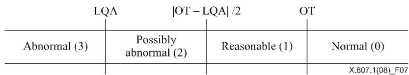
Figure 7 – Mapping of the measured value to a status value
