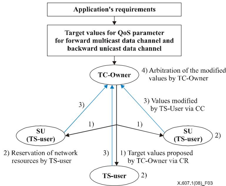
**Figure 3 – QoS negotiation in the ECTP duplex connection**
