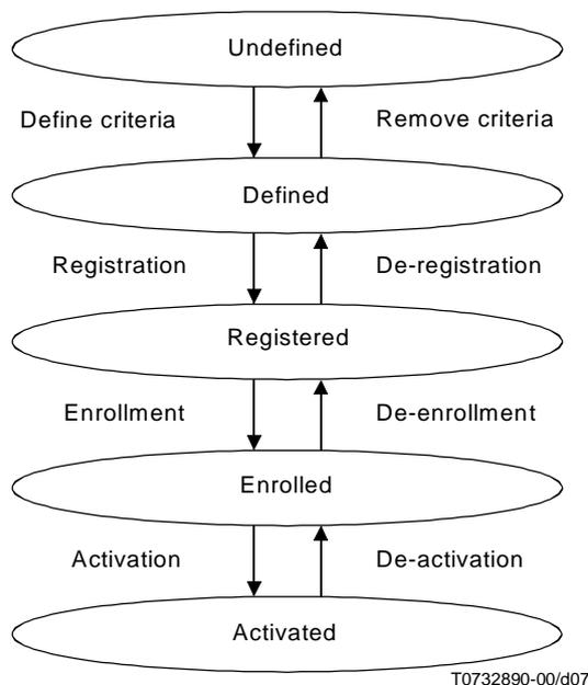
**Figure 7/X.601 – State transition diagram of a group member**
