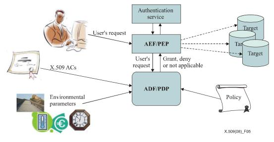
Figure 5 – The control model for a single domain PMI
