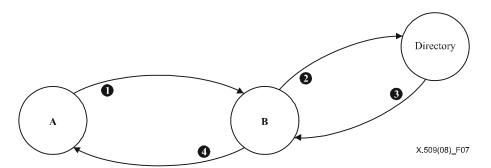
Figure 7 – The unprotected simple authentication procedure
