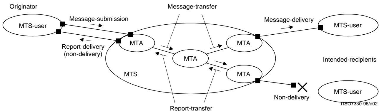
Figure 3 – Refined Message Transfer System model
