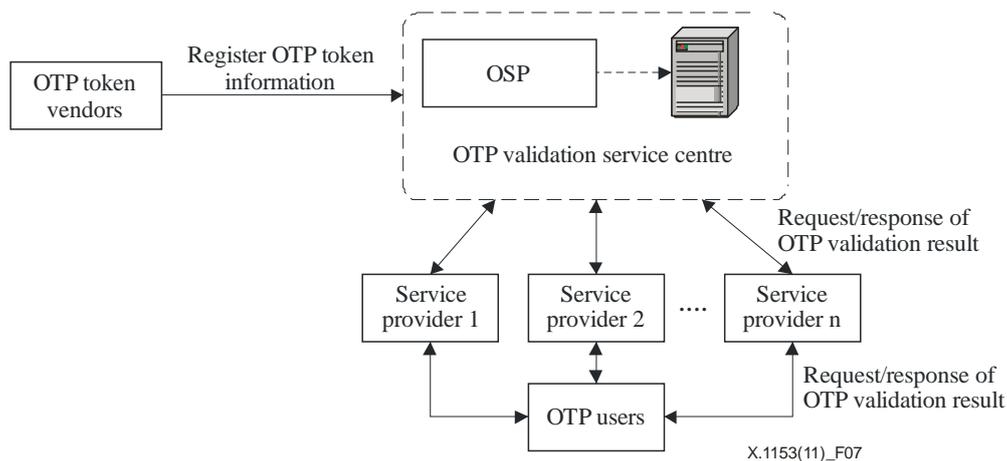
**Figure 7 – OTP management model for the centralized management framework**
