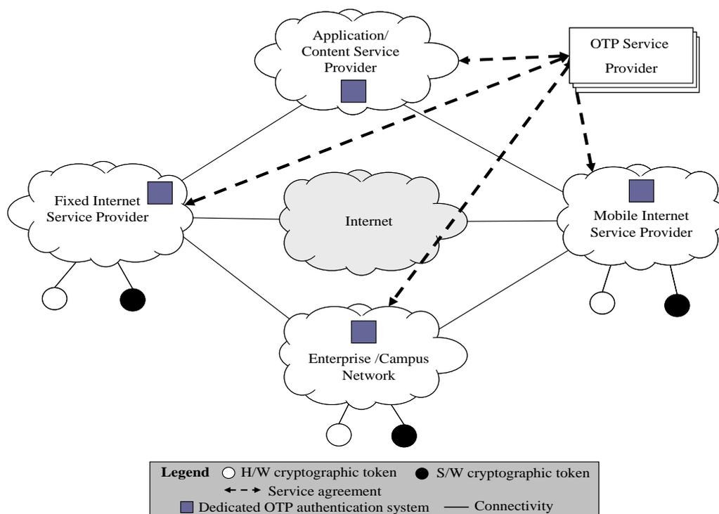
**Figure 4 – Overview of the OTP-based authentication service in multiple service domains**
