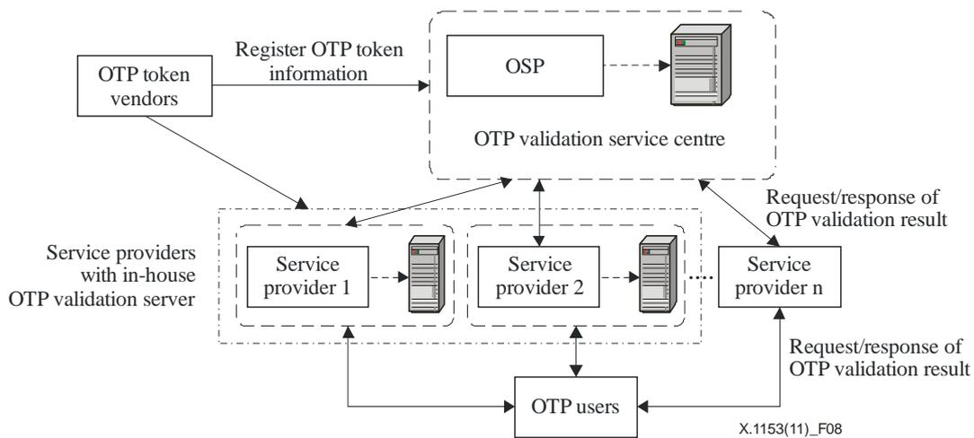
**Figure 8 – OTP management model for the enhanced centralized management framework**
