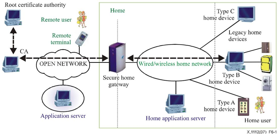
**Figure 6-1 – Device authentication model for the secure home network**
