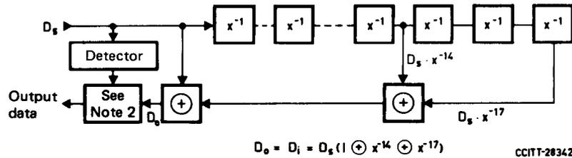
Note 1 - Marks (binary 1) and spaces (binary 0) at the V.24 interface correspond to ones and zeros, respectively, in this logic diagram.
