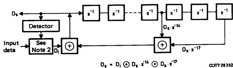
Note 1 Marks (binary 1) and spaces (binary 0) at the V.24 interface correspond to ones and zeros, respectively, in this logic diagram.
