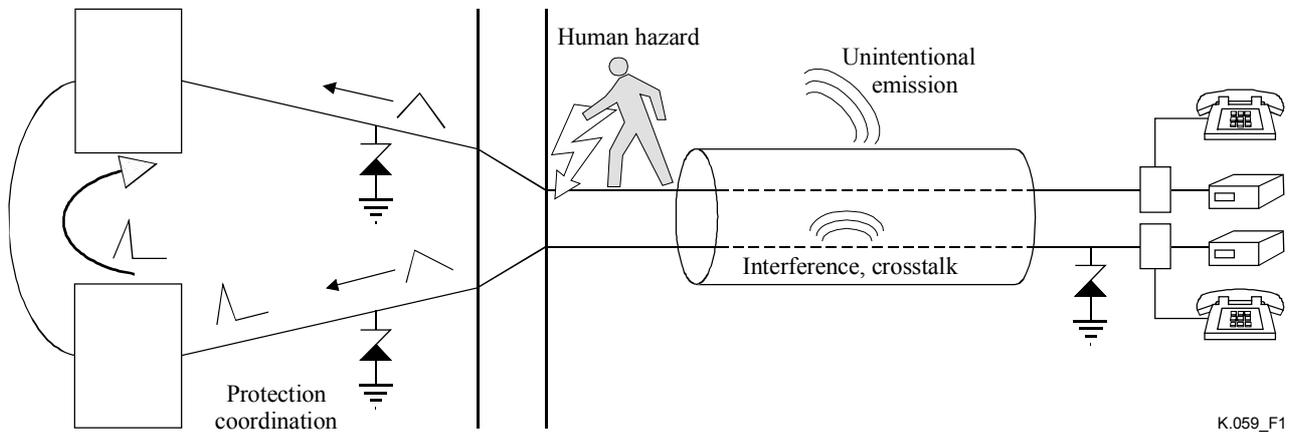
**Figure 1/K.59 – Configuration and problems for unbundled cable**
