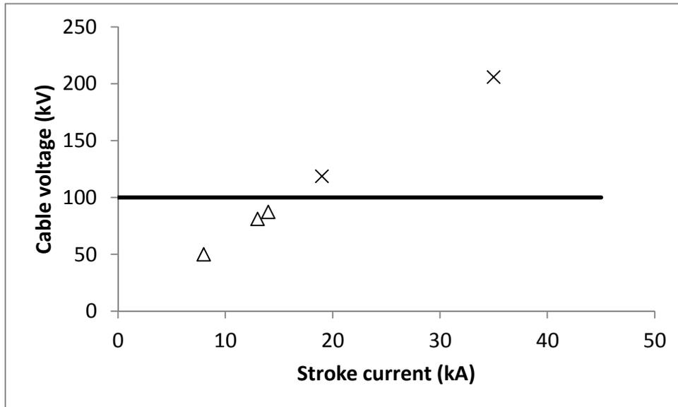
NOTE –  $\Delta$ : strokes that did not break down the cable insulation;  $\times$ : strokes that did break down the cable insulation.
