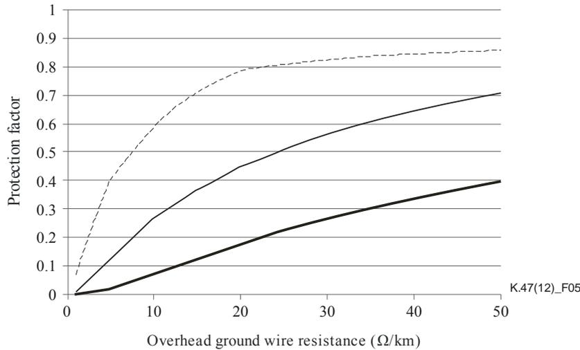
NOTE –  $U_b = 100$  kV;  $l_t = 50$  m; bold line:  $R_t = 10 \Omega$ ; thin line:  $R_t = 30 \Omega$ ; dashed line:  $R_t = 100 \Omega$ .
