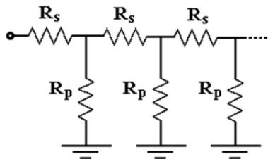
Figure II.1 – Resistive model for the guard-wire
