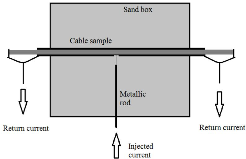
**Figure B.1 – Diagram of the test set up**
