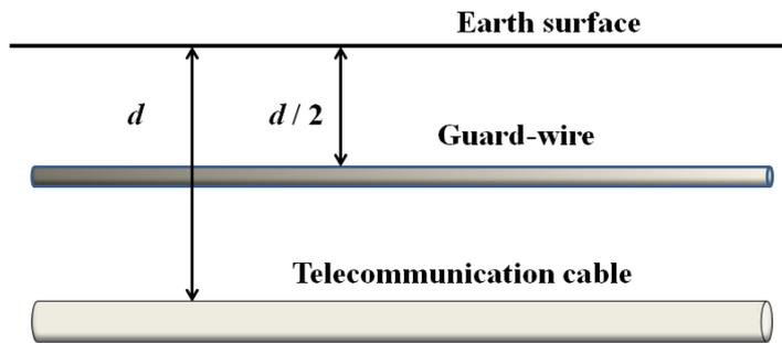
**Figure 3 – Typical guard-wire installation**
