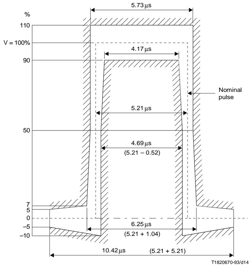
NOTE – For clarity of presentation, the above values are based on a pulse width of 5.21  $\mu$ s. See 8.1 for a precise specification of the bit rate.
