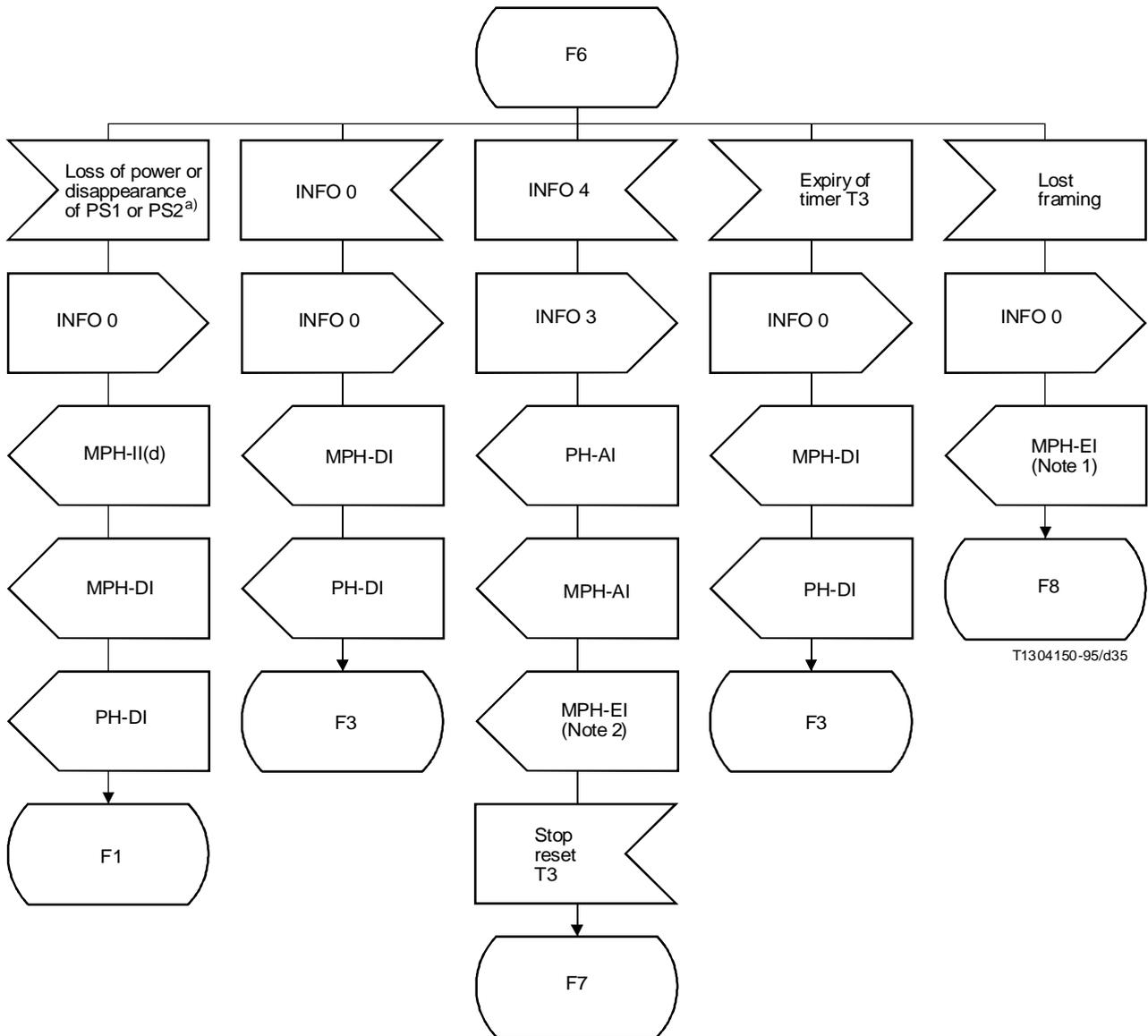
a) Whichever power source is used for determining the connection status.
