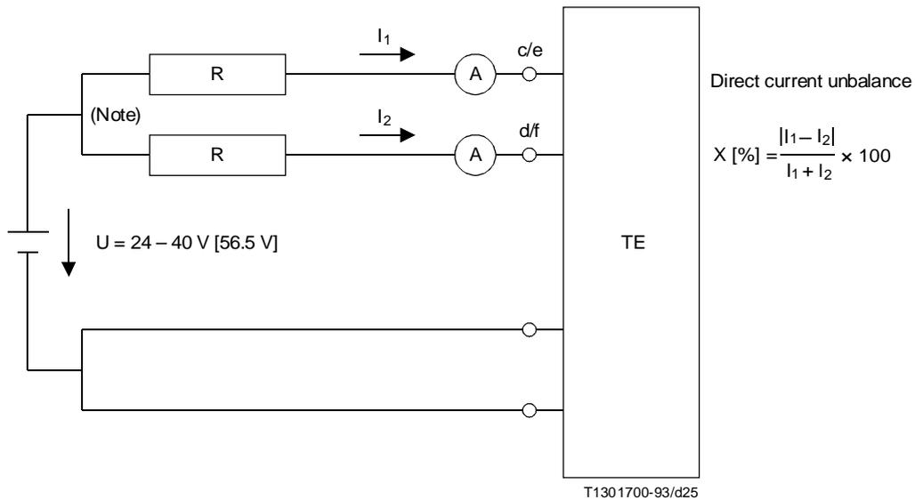
NOTE – The resistors R (2 ohm) represent the TE cord equivalent. They should not be used if the TE has an attached cord.
