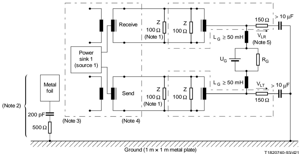
$V_{LT}$  and  $V_{LR} \leq -24$  dBV peak.
