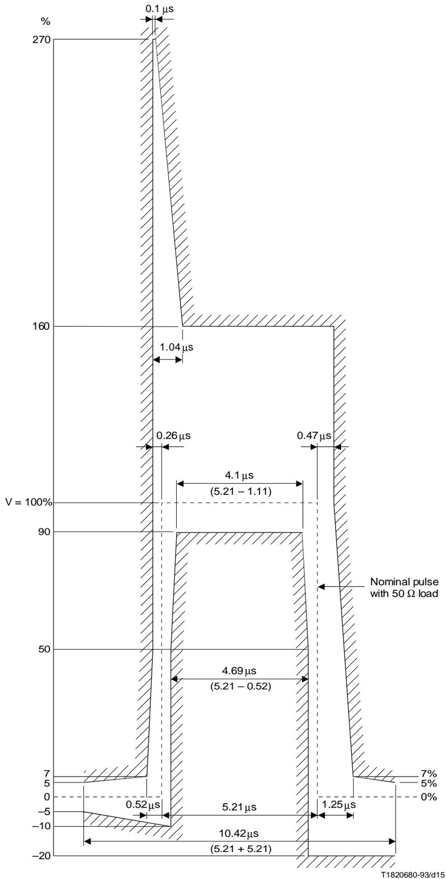
NOTE – For clarity of presentation, the above values are based on a pulse width of 5.21  $\mu\text{s}$ . See 8.1 for a precise specification of the bit rate.
