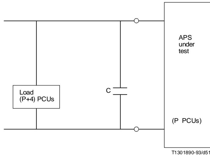
C Capacitor with value  $(P \times 10 \mu\text{F})$
