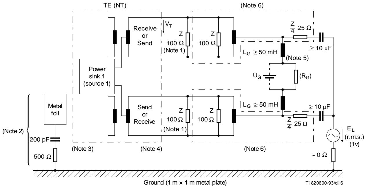
The longitudinal conversion loss:  $LCL = 20 \log_{10} \left| \frac{E_L}{V_L} \right|$  dB.
