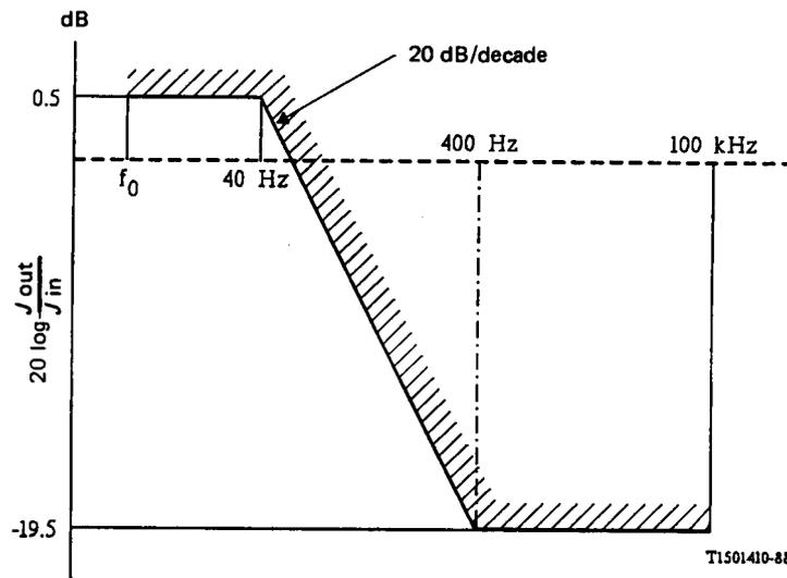
*Note 1* - The frequency  $f_0$  should be less than 20 Hz and as low as possible (e.g. 10 Hz), taking into account the limitations of measuring equipment.
