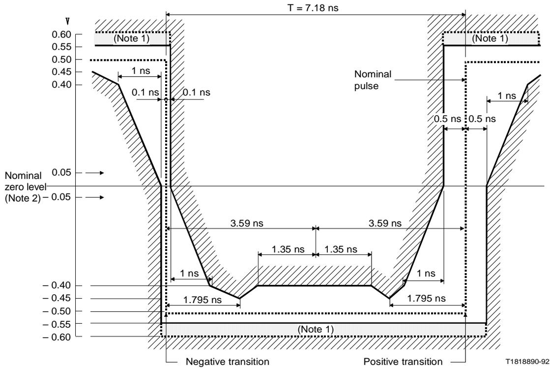
*Note 1* – The maximum "steady state" amplitude should not exceed the 0.55 V limit. Overshoots and other transients are permitted to fall into the dotted area, bounded by the amplitude levels 0.55 V and 0.6 V, provided that they do not exceed the steady state level by more than 0.05 V. The possibility of relaxing the amount by which the overshoot may exceed the steady state level is under study.
