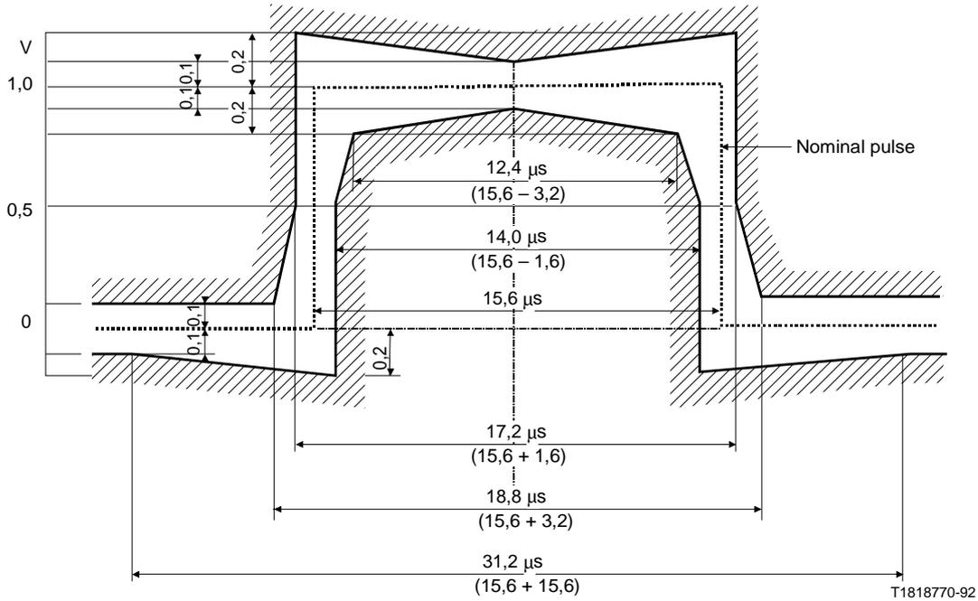
*Note 1* – When one pulse is immediately followed by another pulse of the opposite polarity, the time limits at the zero-crossing between the pulses should be  $\pm 0.8 \mu\text{s}$ .
