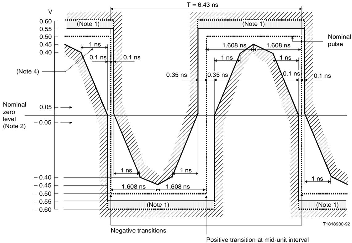
*Note 1* – The maximum "steady state" amplitude should not exceed the 0.55 V limit. Overshoots and other transients are permitted to fall into the dotted area, bounded by the amplitude levels 0.55 V and 0.6 V, provided that they do not exceed the steady state level by more than 0.05 V. The possibility of relaxing the amount by which the overshoot may exceed the steady state level is under study.
