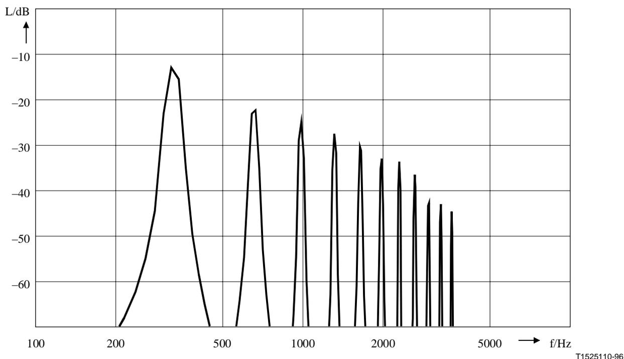
**Figure C.3/G.168 – Power density spectrum of the bandlimited voiced signal (single talk signal, analysis window: Hanning)**
