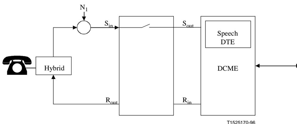
Figure I.3/G.168 – Speech detector/echo control device interaction
