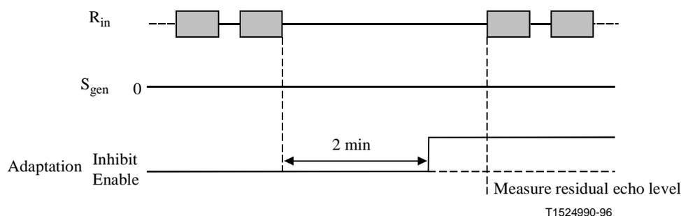
Figure 13/G.168 – Test No. 4 signal and time relationships
