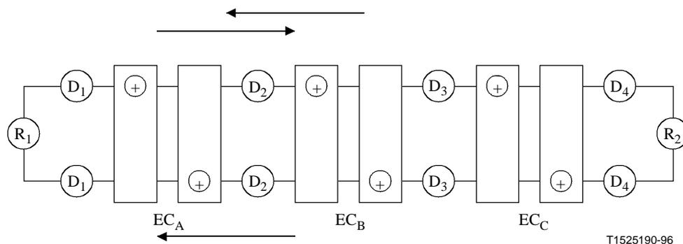
Figure I.2/G.168 – Reference connection for tandem ECs
