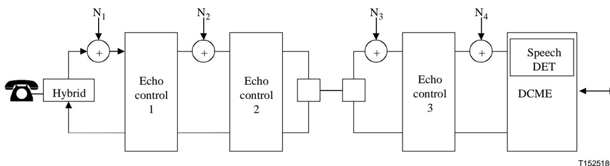
**Figure I.4/G.168 – Multiple echo control devices in a DCME/PCME network configuration**
