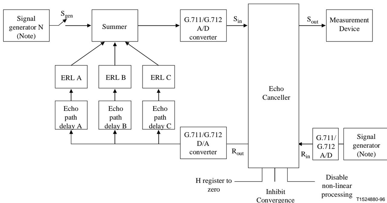
NOTE – The sum of the absolute values of the gains  $G_A$ ,  $G_B$ ,  $G_C$  that correspond to ERL A, B, C, respectively, taken in dB, should be less than or equal to  $-6$  dB (i.e.  $20 \log(|G_A| + |G_B| + |G_C|) \leq -6$  dB), and echo path delay  $A \leq \Delta$  ms, echo path delay  $B \leq \Delta$  ms, and echo path delay  $C \leq \Delta$  ms.
