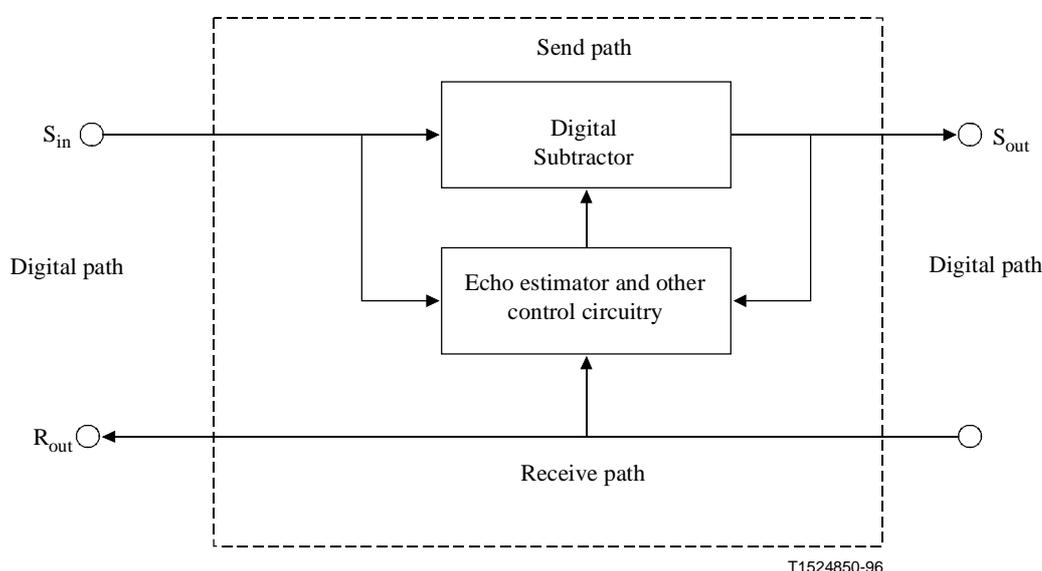
NOTE – Functionally, a Digital Echo Canceller (DEC) interfaces at 64 kbit/s. However, 24 or 30 digital echo cancellers for example may be combined corresponding to the primary digital hierarchy levels of 1544 kbit/s or 2048 kbit/s, respectively.
