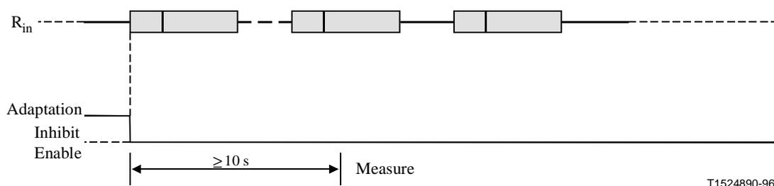
Figure 5/G.168 – Test No. 1 signal and time relationships
