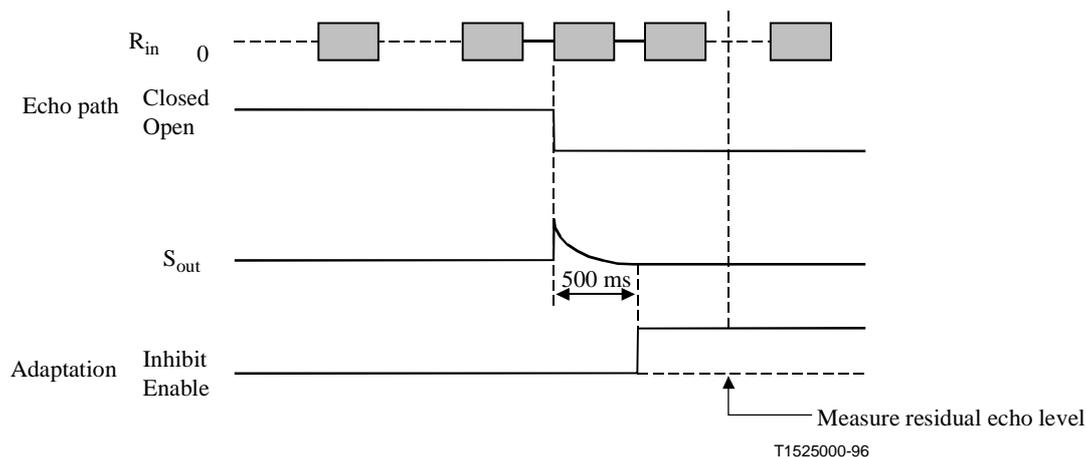
Figure 14/G.168 – Test No. 5 signal and time relationships
