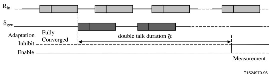
Figure 11/G.168 – Test No. 3B signal and time relationships
