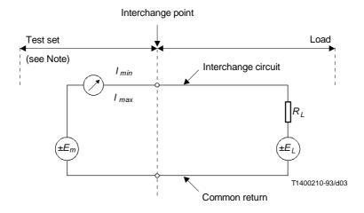
NOTE – The internal resistance of the ammeter shall be much less than the load resistance  $(R_L)$ .
