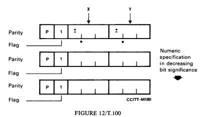
Structure of a block of 3 data bytes
