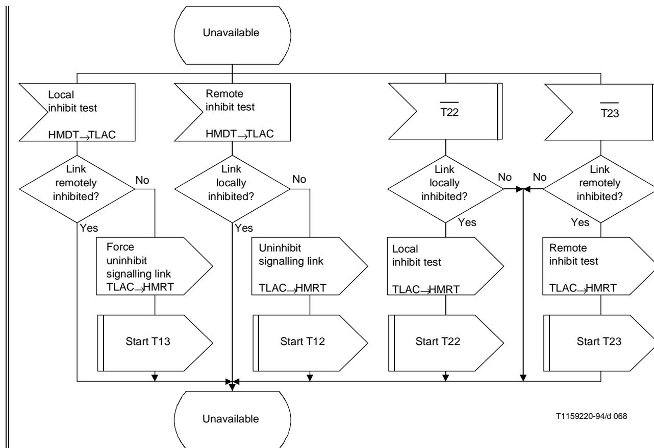
**Figure 28/Q.704 (sheet 15 of 18) – Signalling traffic management; link availability control (TLAC)**
