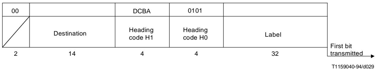
**Figure 20/Q.704 – Signalling-route-set-test message**
