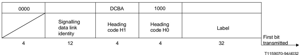
**Figure 22/Q.704 – Signalling-data-link-connection-order message**
