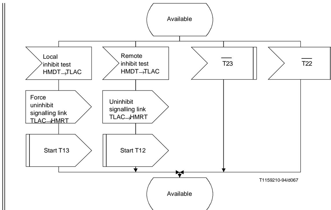
**Figure 28/Q.704 (sheet 14 of 18) – Signalling traffic management; link availability control (TLAC)**
