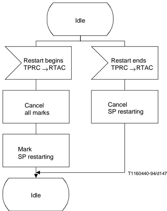
**Figure 45/Q.704 (sheet 2 of 2) – Signalling route management; transfer allowed control (RTAC)**
