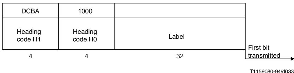
**Figure 22a/Q.704 – Signalling-data-link-connection-acknowledgement message**
