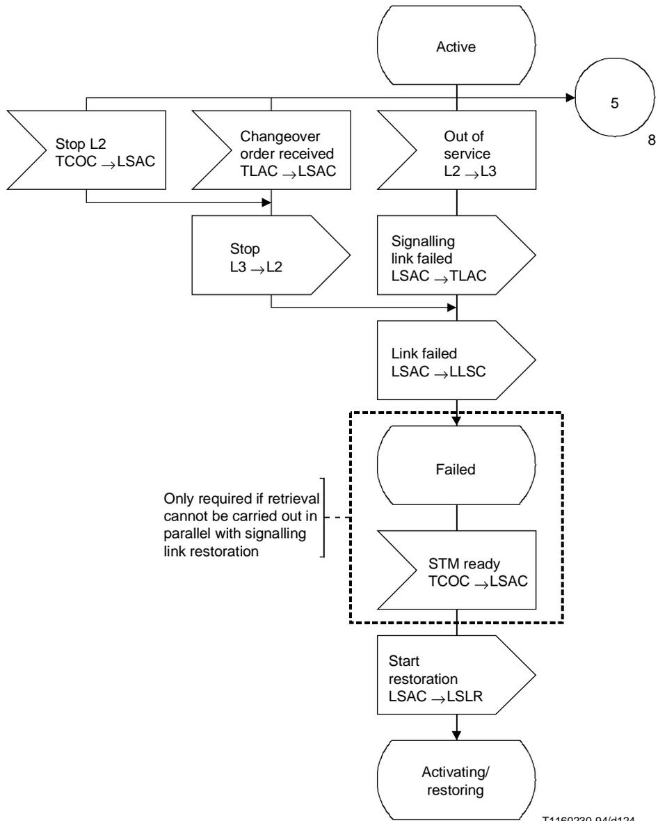
**Figure 37/Q.704 (sheet 7 of 10) – Signalling link management; signalling link activity control (LSAC)**
