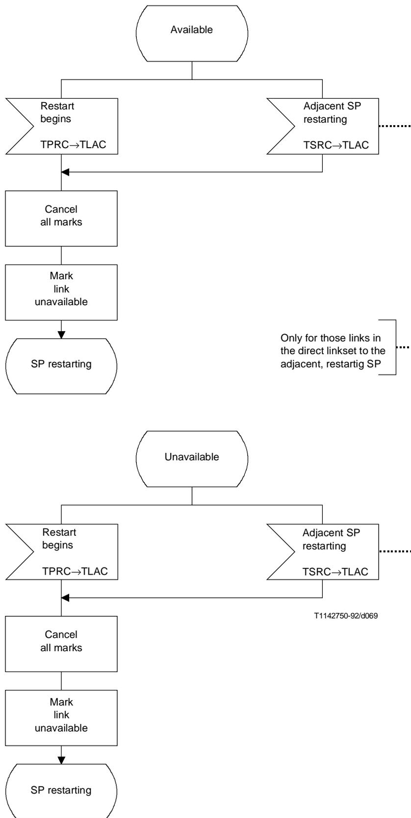
**Figure 28/Q.704 (sheet 16 of 18) – Signalling traffic management; link availability control (TLAC)**
