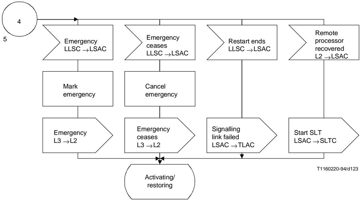
**Figure 37/Q.704 (sheet 6 of 10) – Signalling link management;
