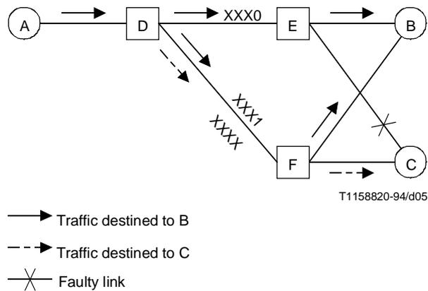
**Figure 5/Q.704 – Example of load sharing between link sets**
