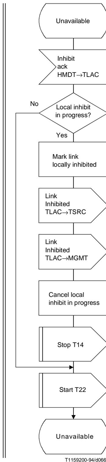
**Figure 28/Q.704 (sheet 13 of 18) – Signalling traffic management;
