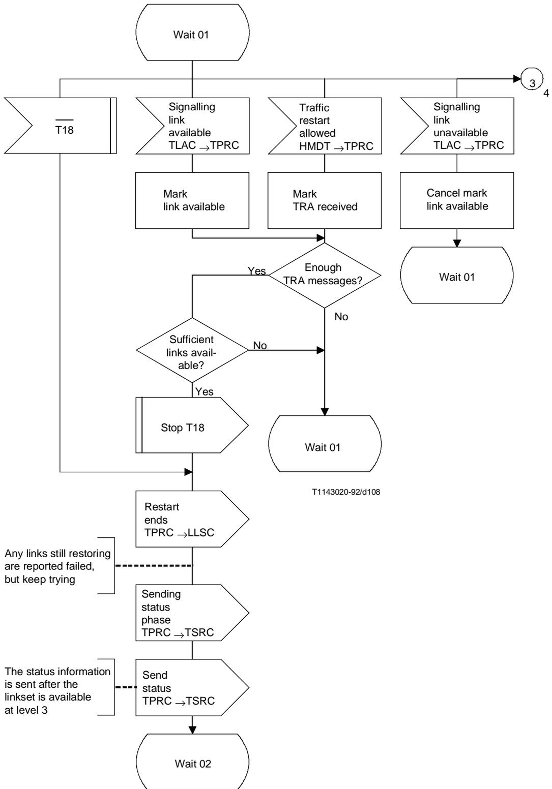
**Figure 34b/Q.704 (sheet 3 of 7) – Signalling traffic management; signalling point restart control (TPRC)**
