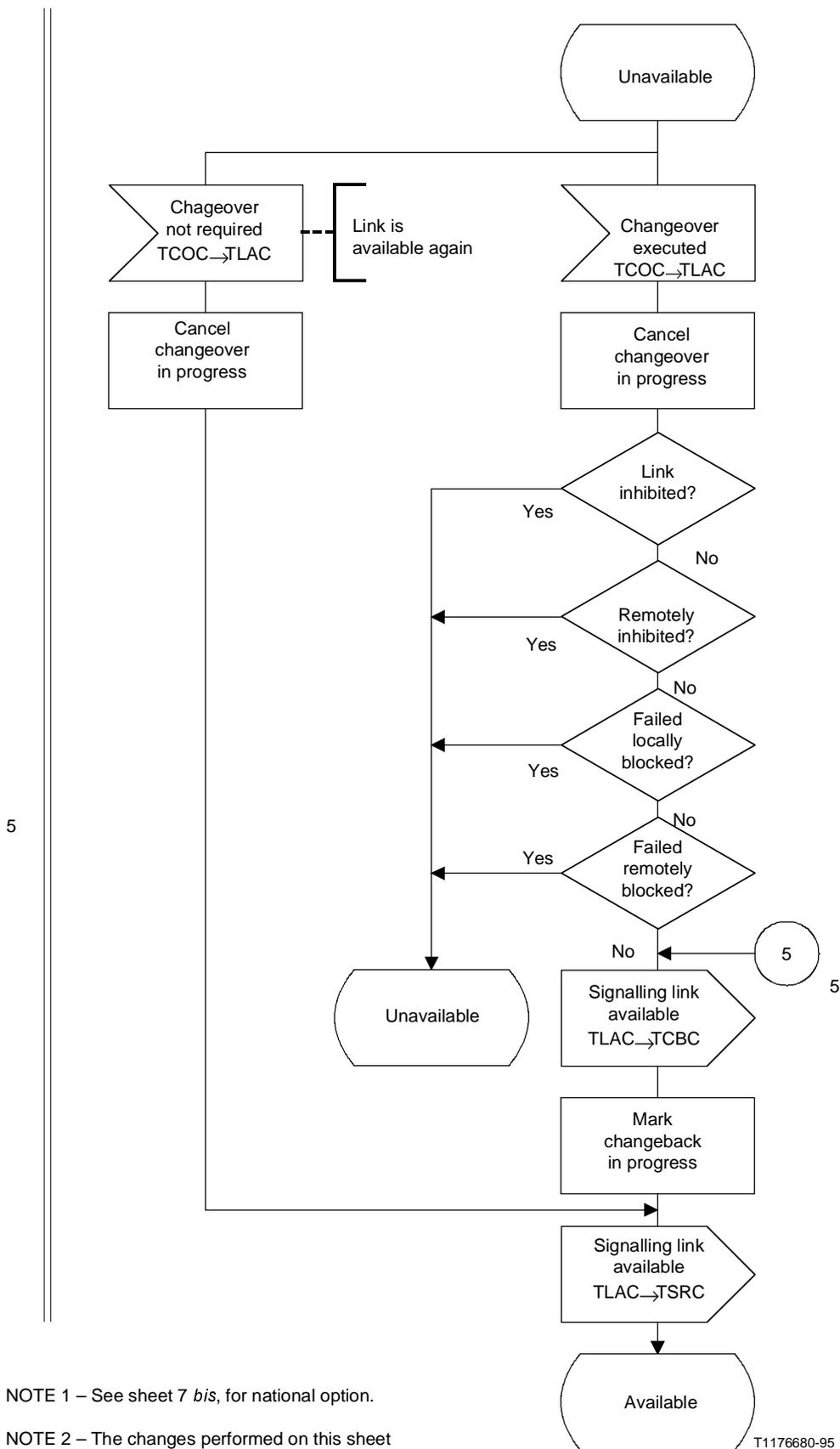
**Figure 28/Q.704 (sheet 7 of 18) – Signalling traffic management; link availability control (TLAC)**
