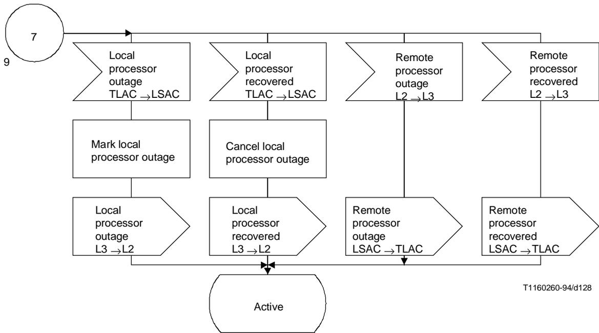
**Figure 37/Q.704 (sheet 10 bis of 10) – Signalling link management;
