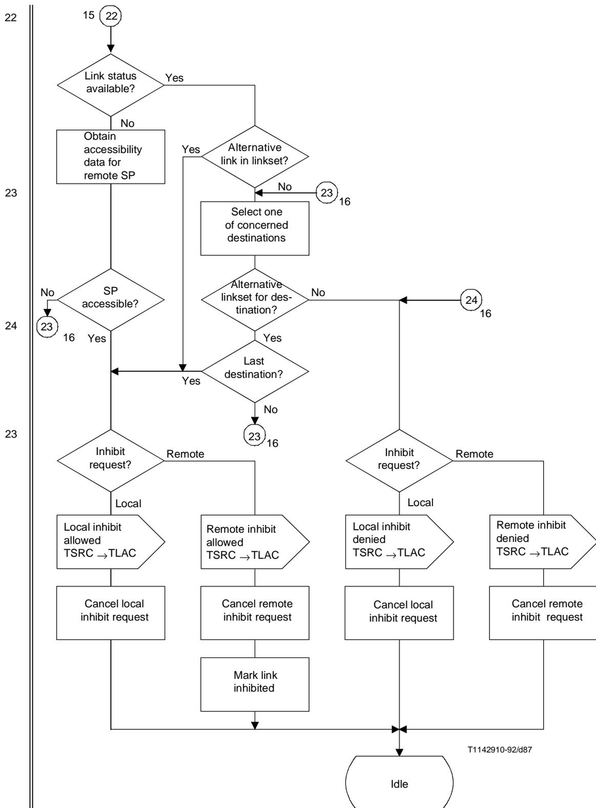
**Figure 29/Q.704 (sheet 16 of 21) – Signalling traffic management; signalling routing control (TSRC)**
