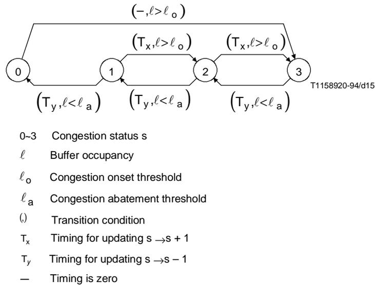
**Figure 8d/Q.704 – An example of signalling link congestion status (using multiple signalling link congestion states without congestion priority)**
