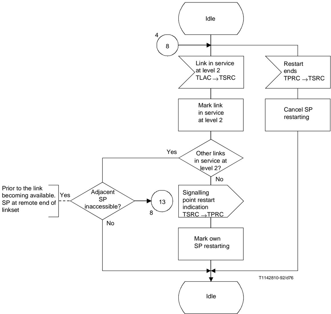
**Figure 29/Q.704 (sheet 5 of 21) – Signalling traffic management; signalling routing control (TSRC)**
