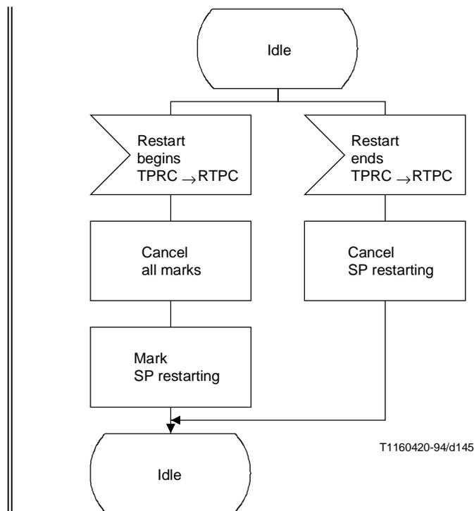
**Figure 44/Q.704 (sheet 3 of 3) – Signalling route management;
