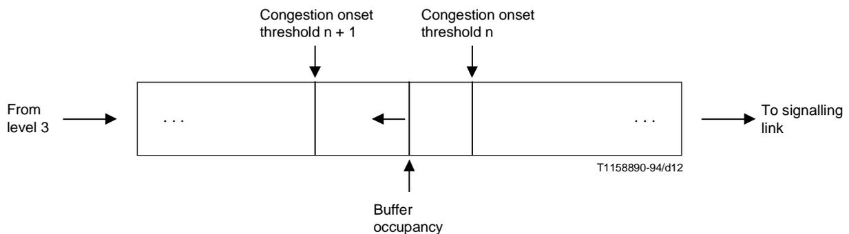
**Figure 8a/Q.704 – Signalling link congestion status =  $n$  (congestion onset)**
