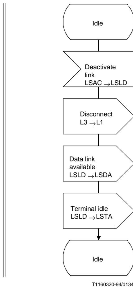
**Figure 40/Q.704 – Signalling link management;
