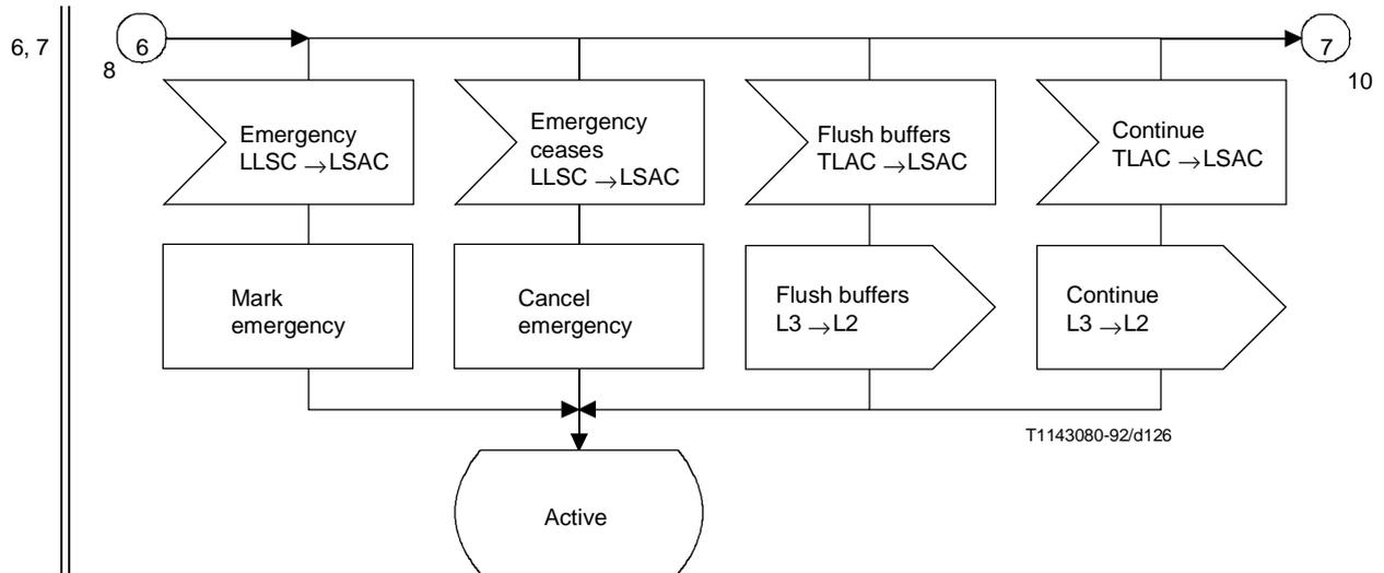
**Figure 37/Q.704 (sheet 9 of 10) – Signalling link management; signalling link activity control (LSAC)**
