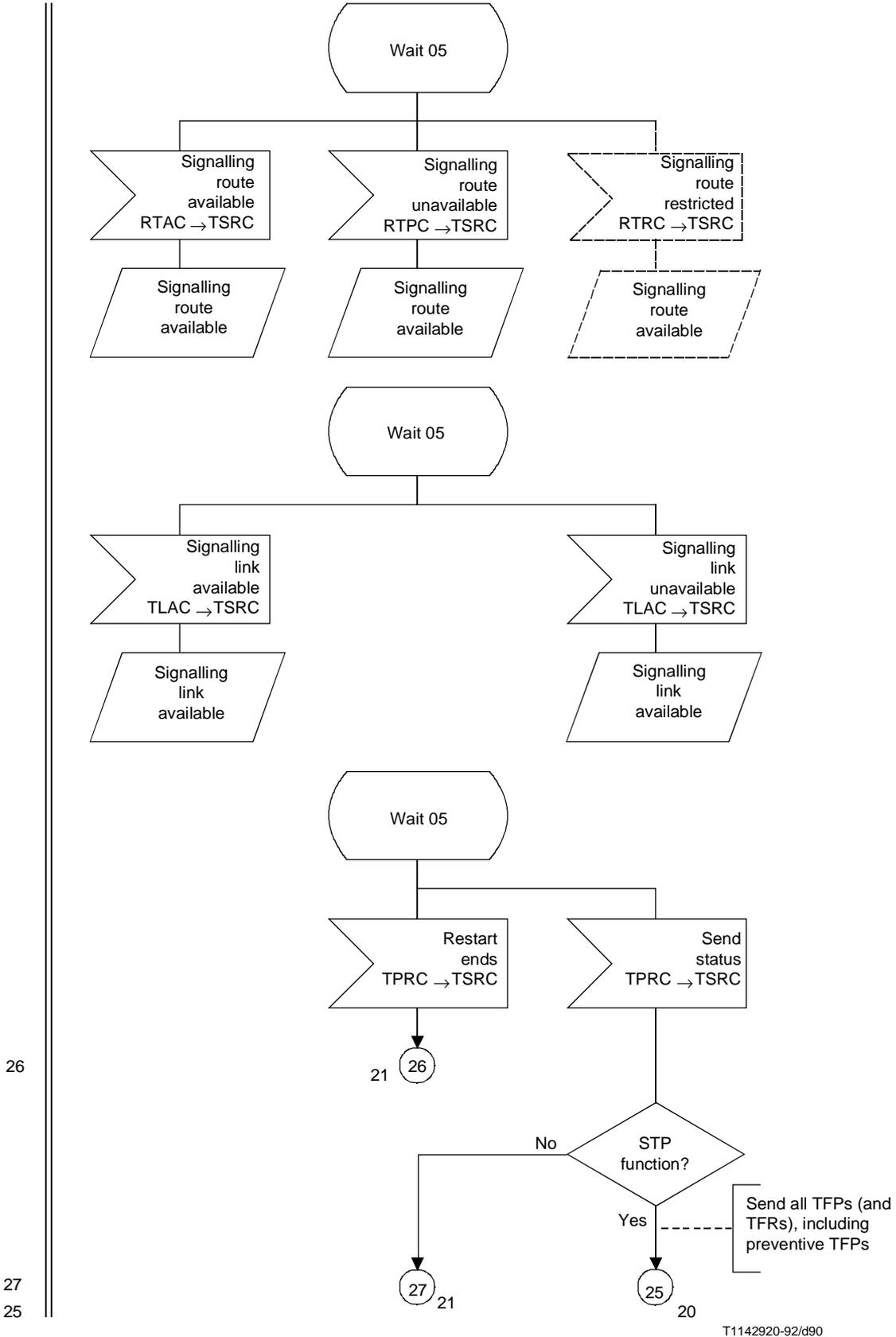
**Figure 29/Q.704 (sheet 19 of 21) – Signalling traffic management; signalling routing control (TSRC)**
