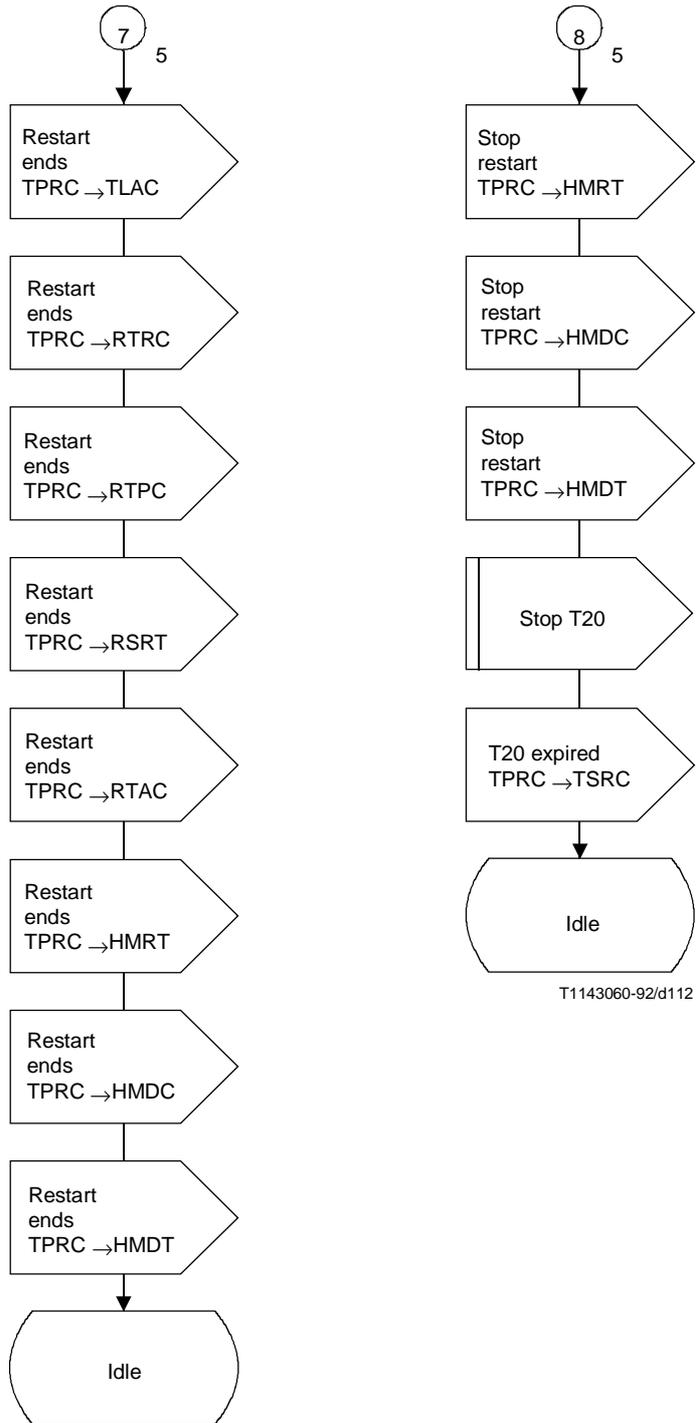
**Figure 34b/Q.704 (sheet 7 of 7) – Signalling traffic management; signalling point restart control (TPRC)**
