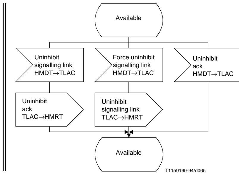
**Figure 28/Q.704 (sheet 12 of 18) – Signalling traffic management;
