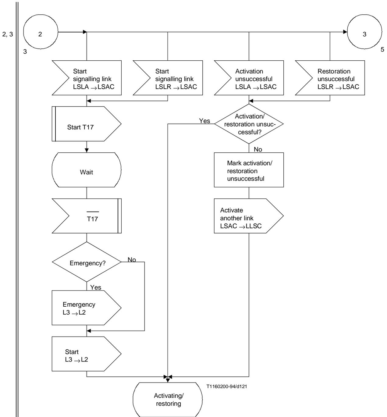
**Figure 37/Q.704 (sheet 4 of 10) – Signalling link management; signalling link activity control (LSAC)**
