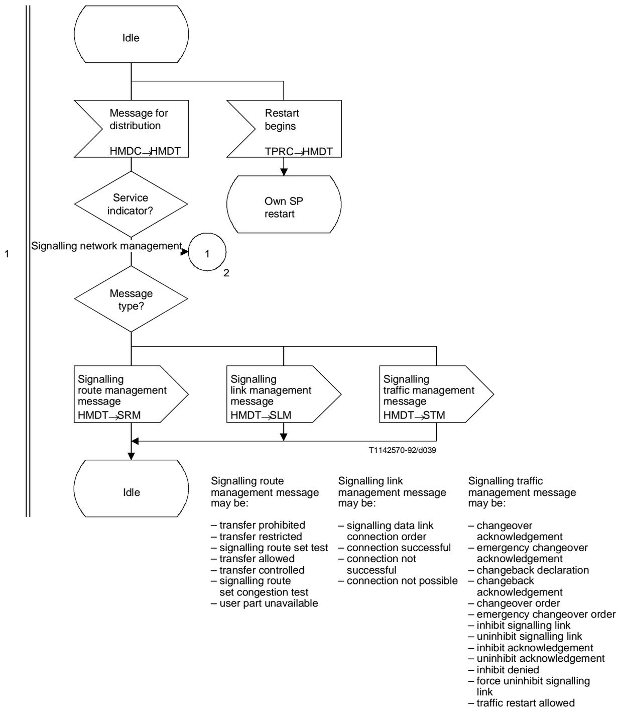
**Figure 25/Q.704 (sheet 1 of 3) – Signalling message handling; message distribution (HMDT)**
