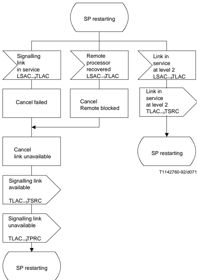
**Figure 28/Q.704 (sheet 18 of 18) – Signalling traffic management; link availability control (TLAC)**
