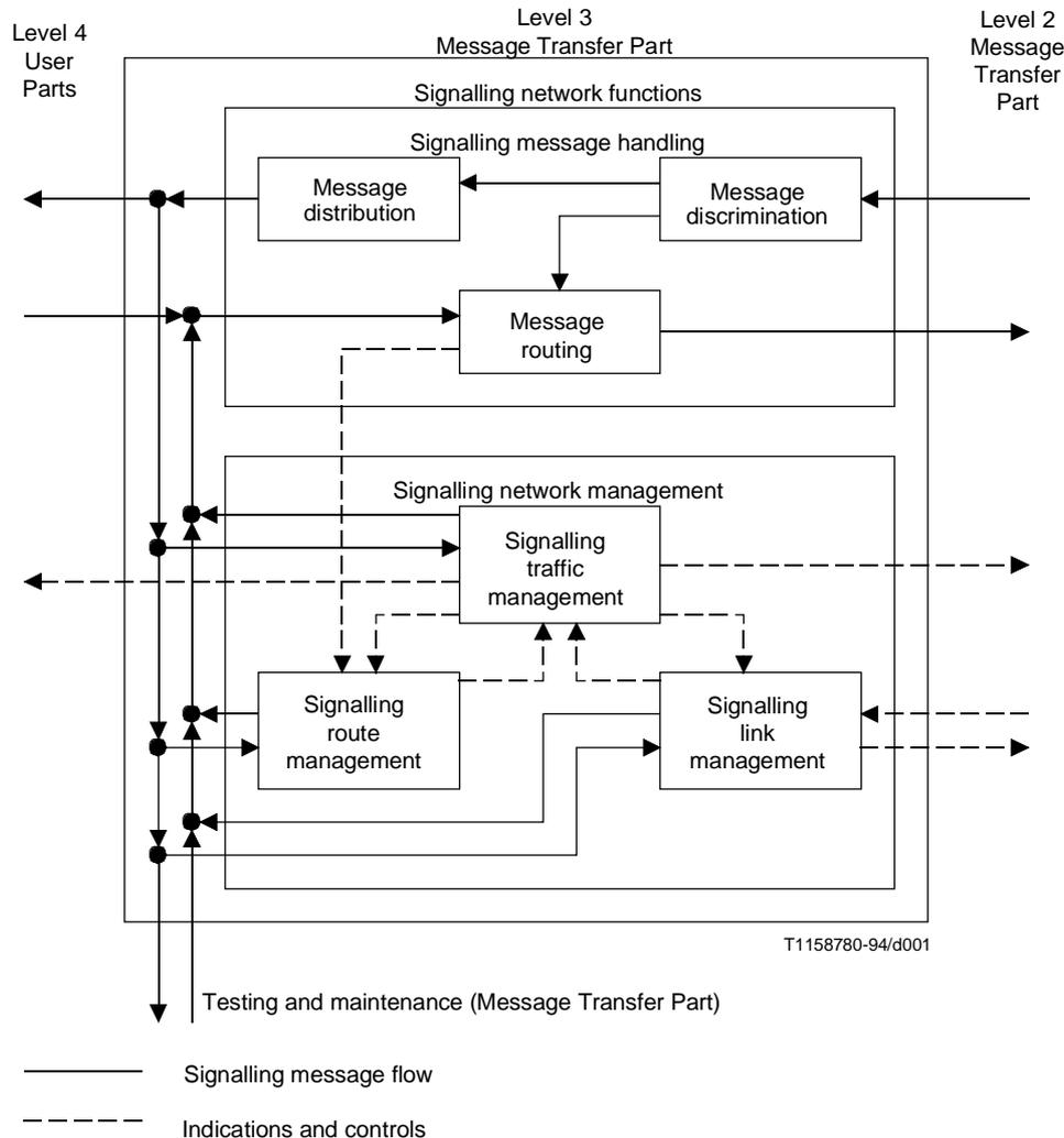
**Figure 1/Q.704 – Signalling network functions**
