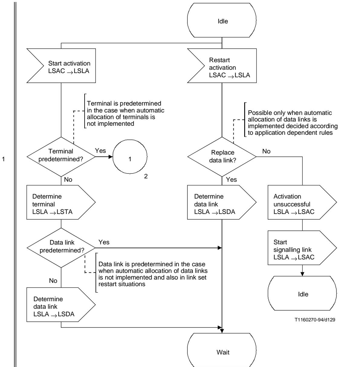
**Figure 38/Q.704 (sheet 1 of 3) – Signalling link management; signalling link activation (LSLA)**
