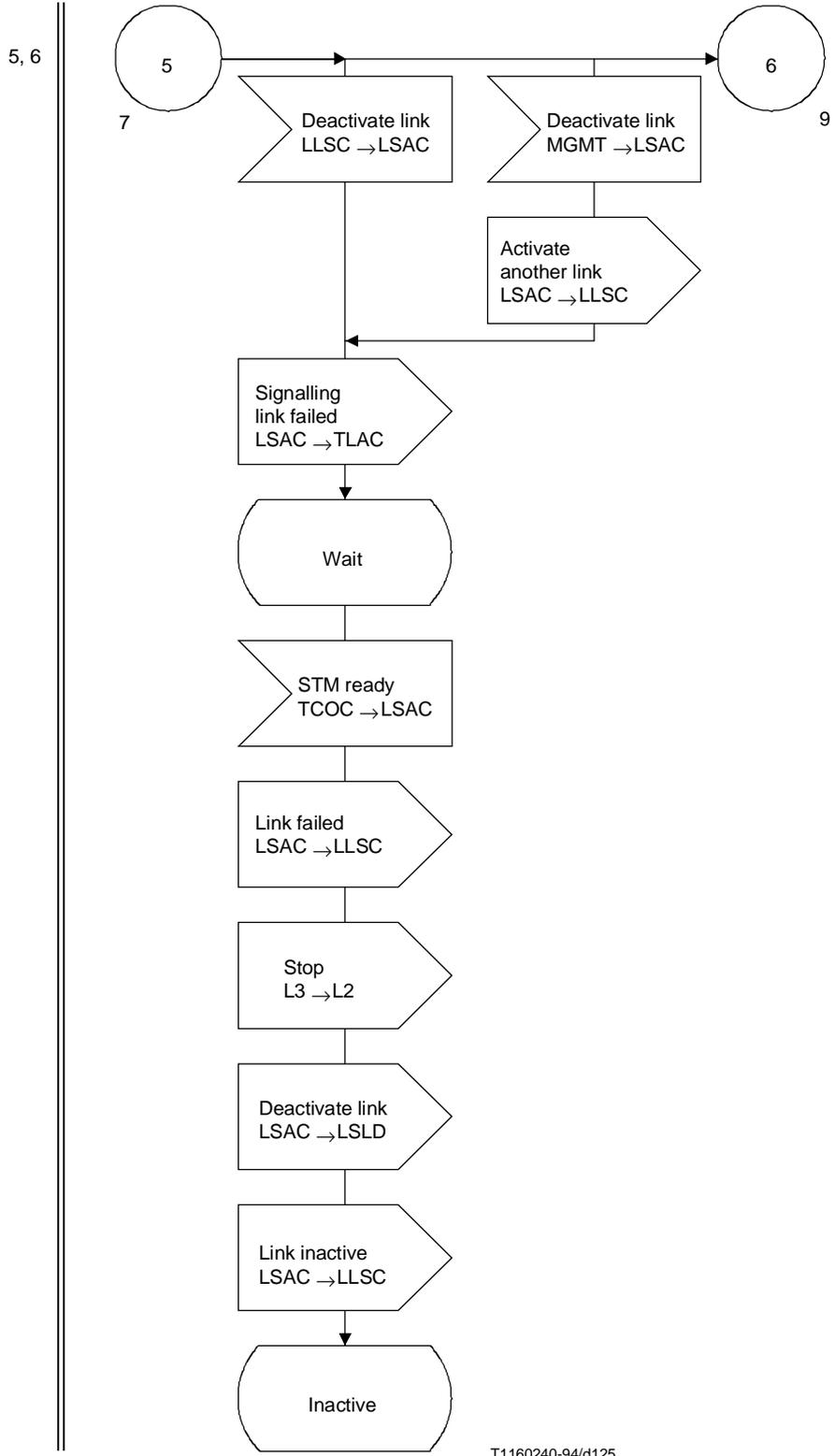
**Figure 37/Q.704 (sheet 8 of 10) – Signalling link management;
