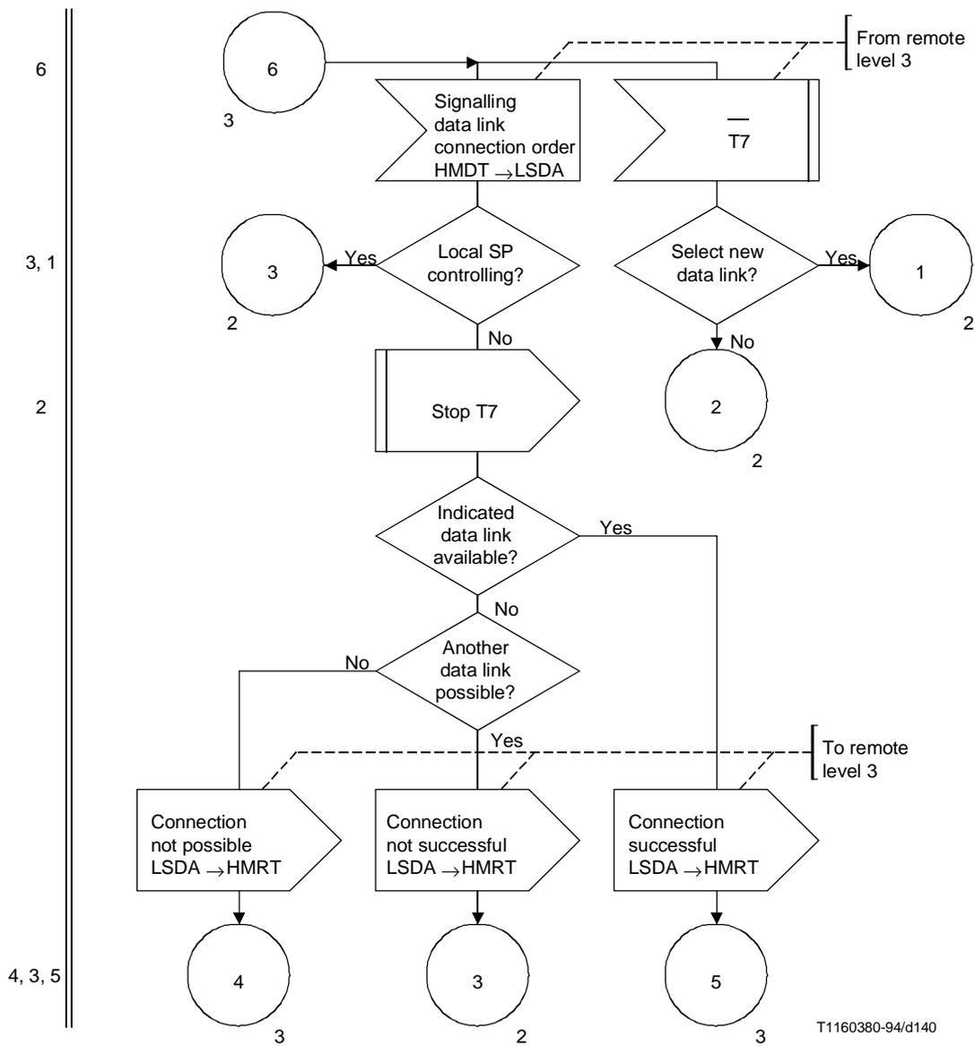
**Figure 42/Q.704 (sheet 4 of 4) – Signalling link management;
