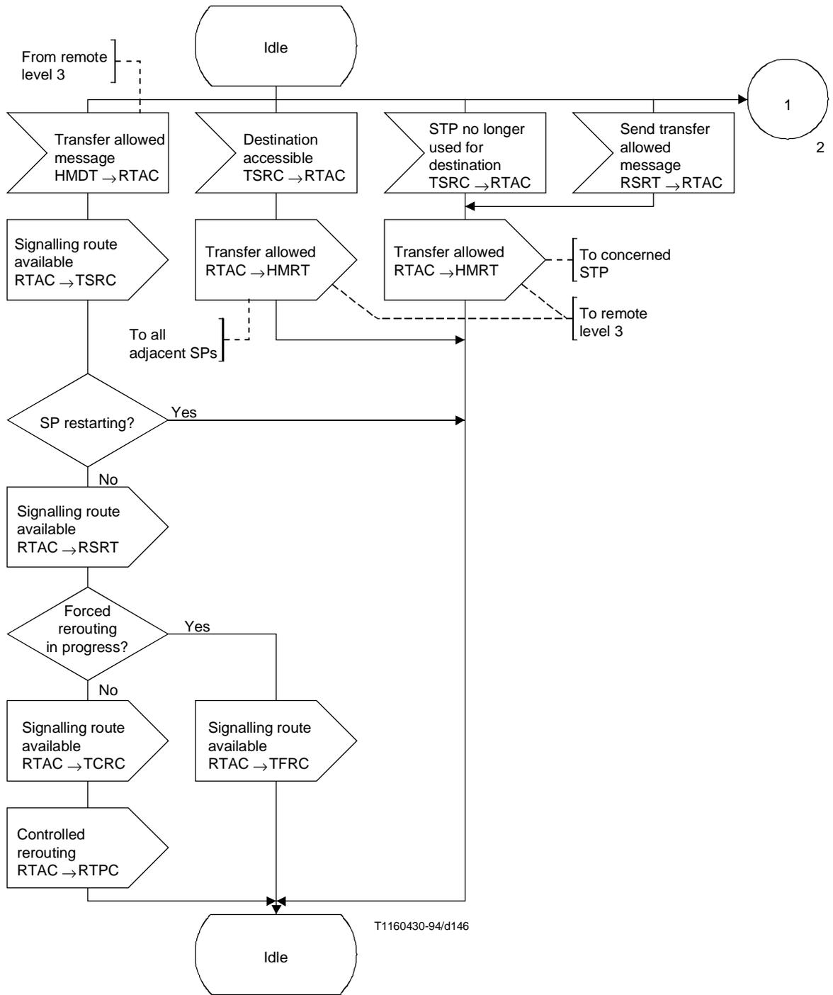
**Figure 45/Q.704 (sheet 1 of 2) – Signalling route management; transfer allowed control (RTAC)**
