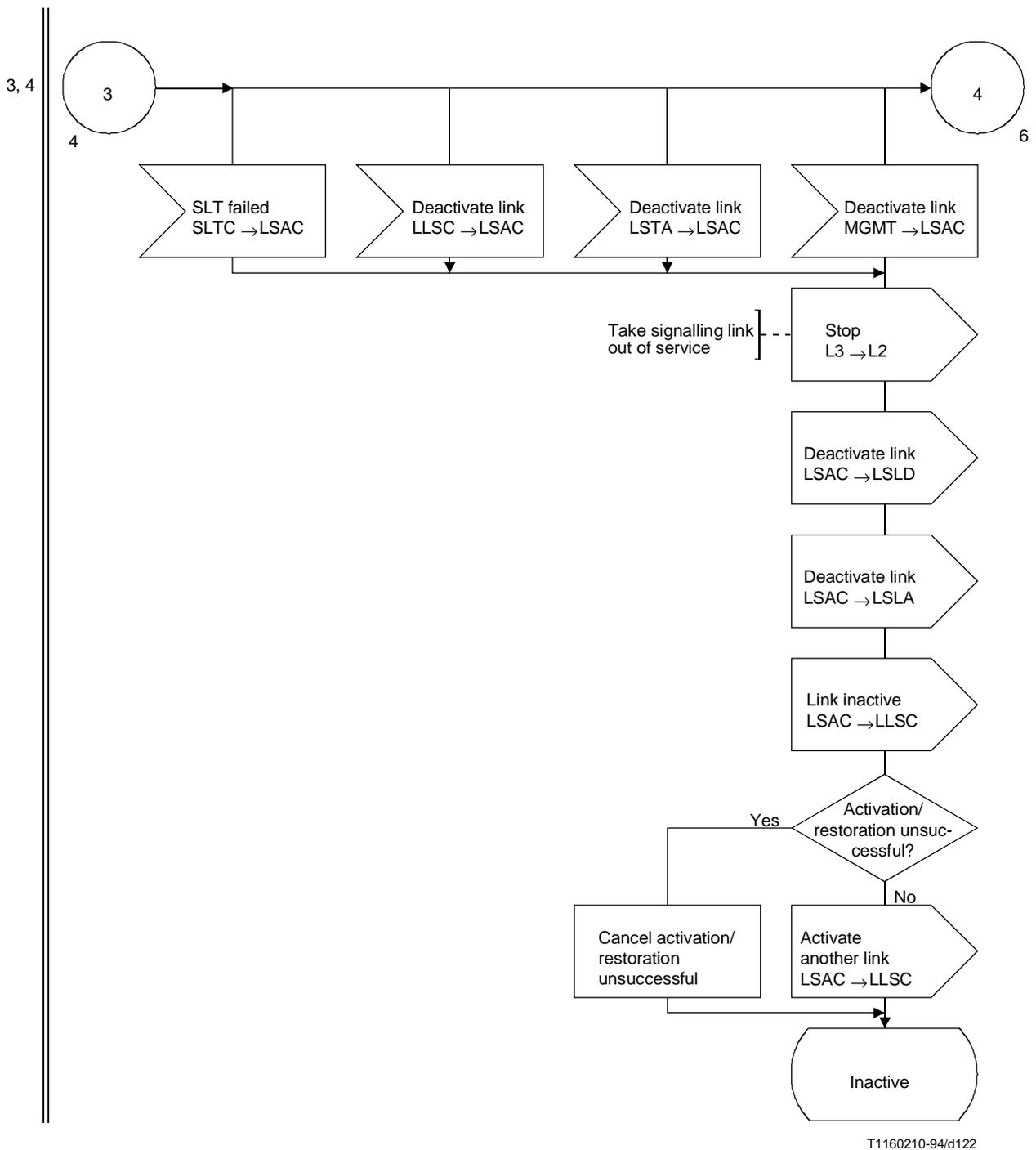
**Figure 37/Q.704 (sheet 5 of 10) – Signalling link management; signalling link activity control (LSAC)**
