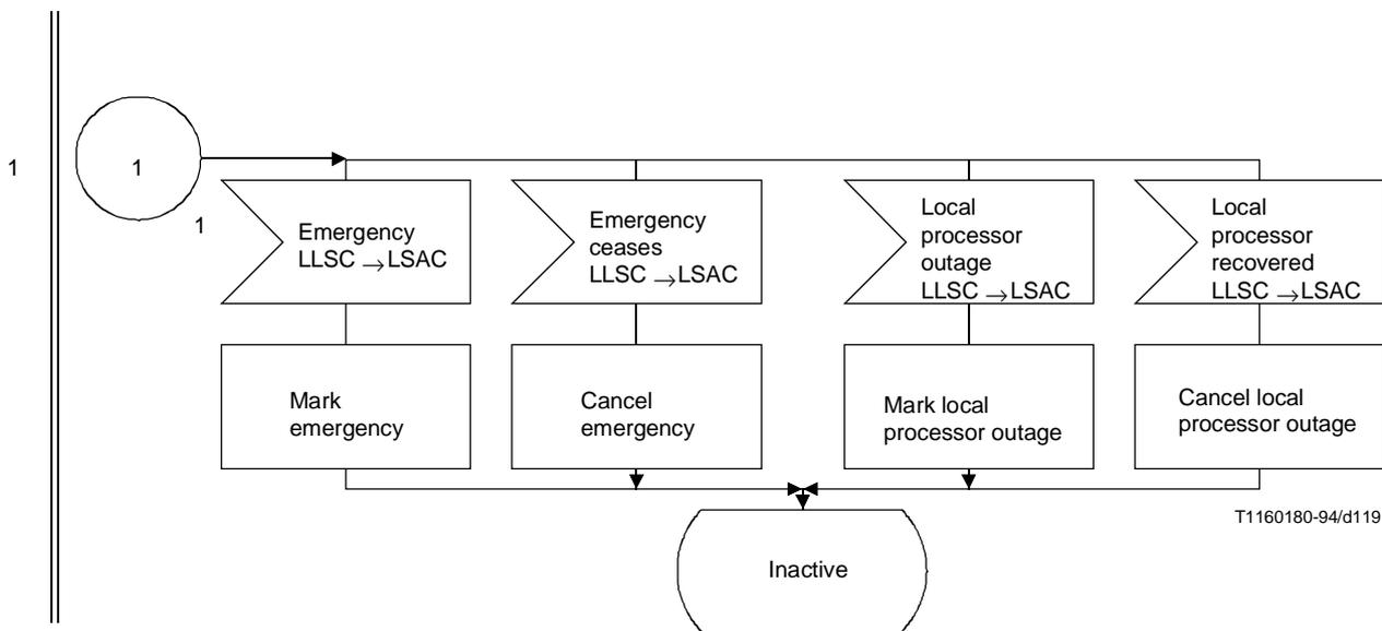
**Figure 37/Q.704 (sheet 2 bis of 10) – Signalling link management; signalling link activity control (LSAC)**
