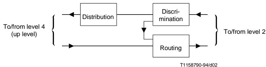
**Figure 2/Q.704 – Message routing, discrimination and distribution**
