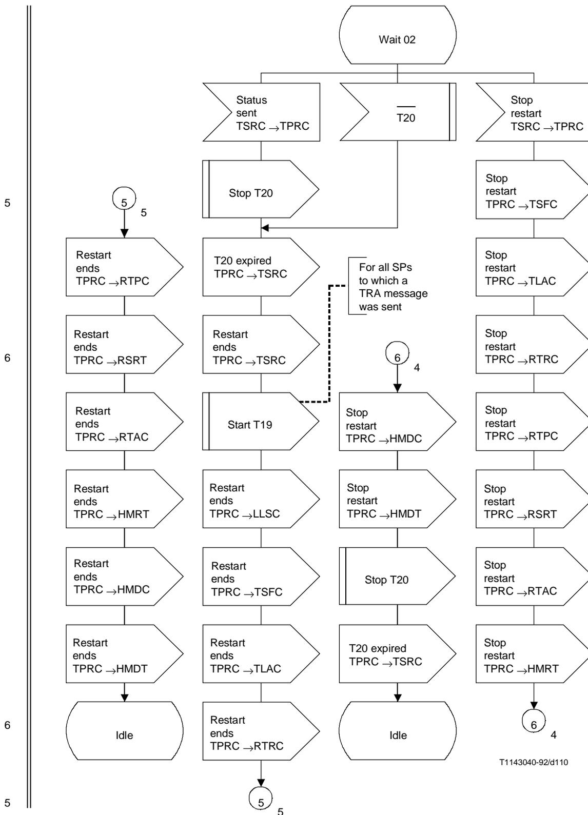
**Figure 34b/Q.704 (sheet 5 of 7) – Signalling traffic management; signalling point restart control (TPRC)**
