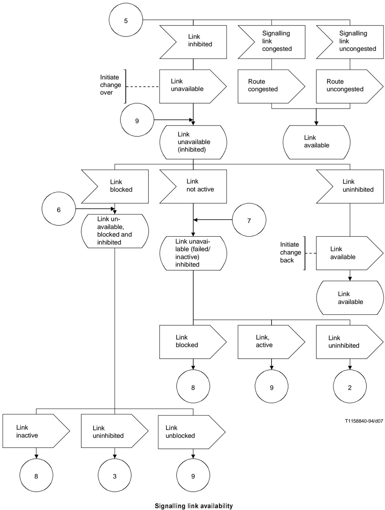
**Figure 6/Q.704 (sheet 2 of 4) – Signalling traffic management overview diagram**
