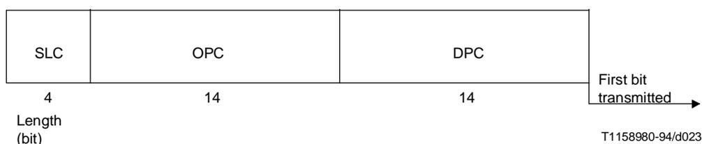
**Figure 14/Q.704 – Standard label structure**
