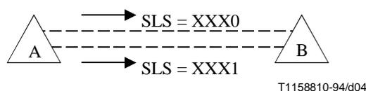
**Figure 4/Q.704 – Example of load sharing within a link set**
