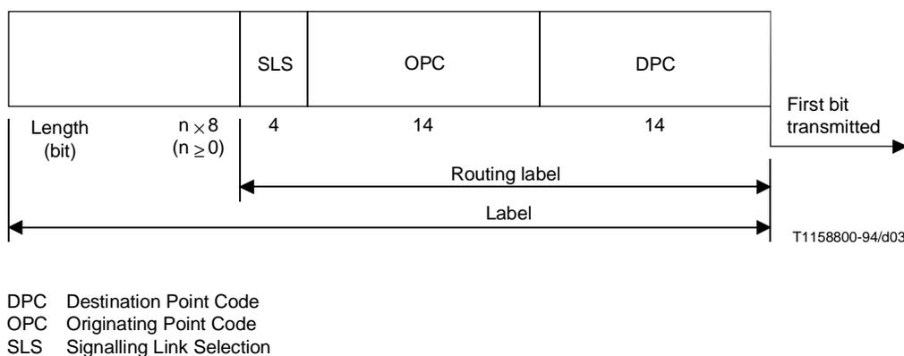
**Figure 3/Q.704 – Routing label structure**
