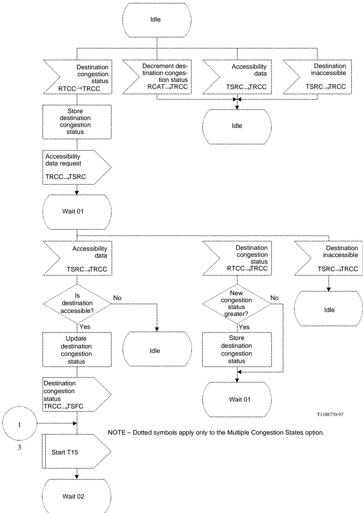
**Figure 29a/Q.704 (sheet 1 of 3) – Signalling traffic management; signalling route set congestion control (TRCC)**
