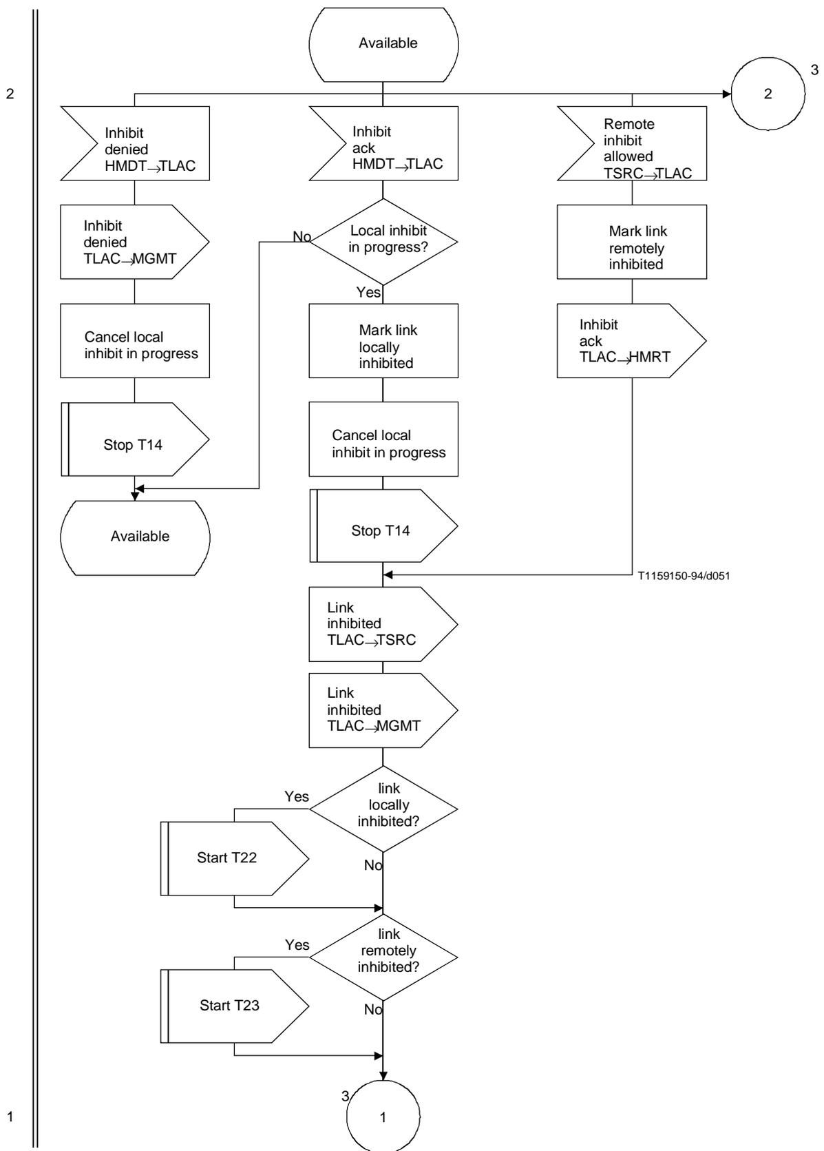
Figure 28/Q.704 (sheet 2 of 18) – Signalling traffic management; link availability control (TLAC)
