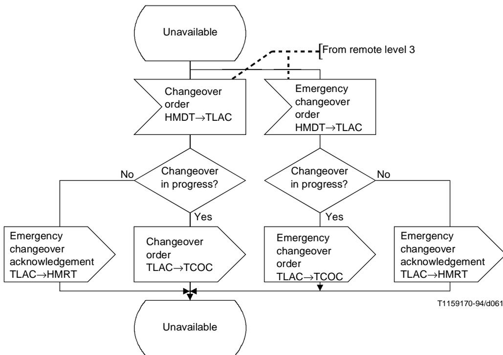
**Figure 28/Q.704 (sheet 8 of 18) – Signalling traffic management;
