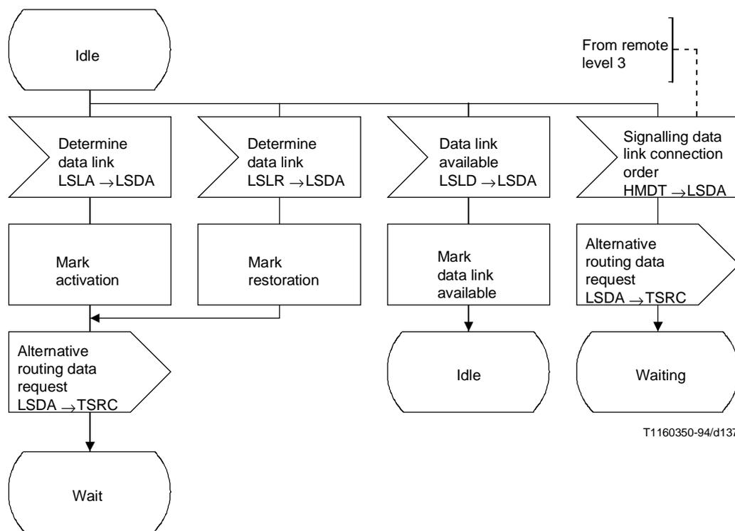
**Figure 42/Q.704 (sheet 1 of 4) – Signalling link management; signalling data link allocation (LSDA)**
