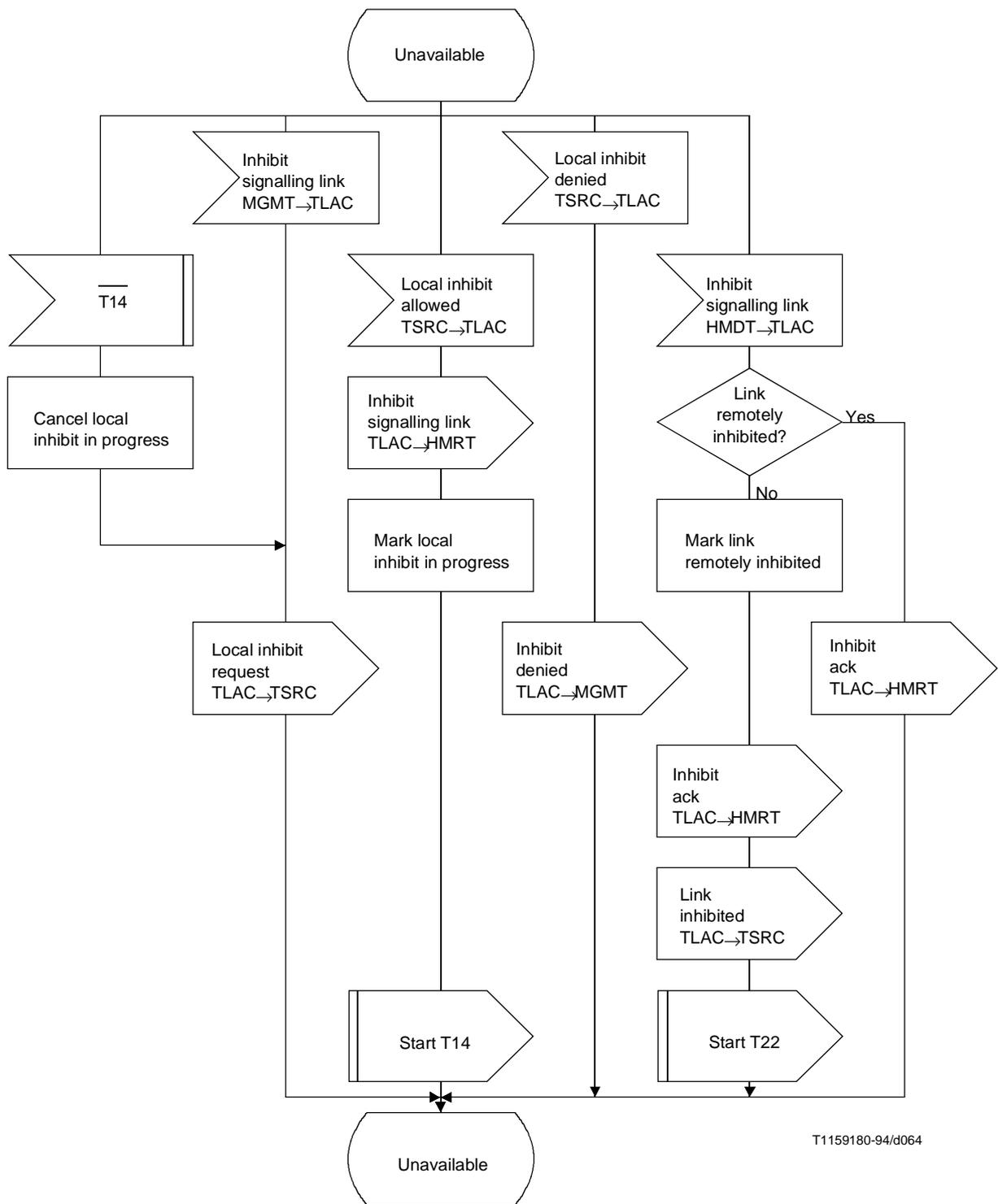
**Figure 28/Q.704 (sheet 11 of 18) – Signalling traffic management; link availability control (TLAC)**
