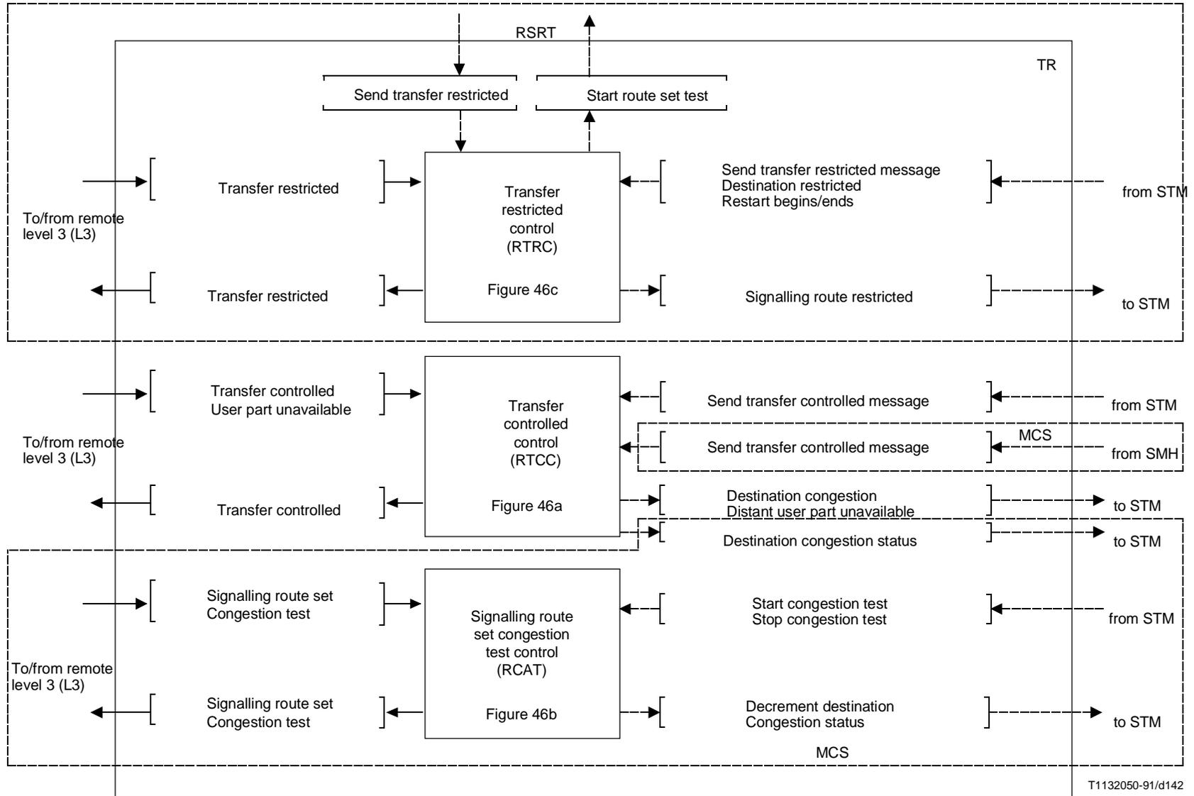
Figure 43/Q.704 (sheet 2 of 2) – Level 3 – Signalling route management (SRM); functional block interactions
