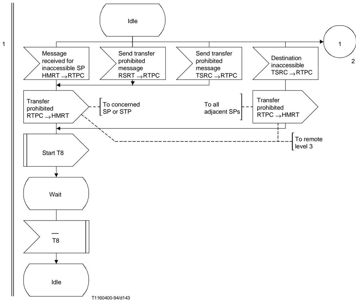
**Figure 44/Q.704 (sheet 1 of 3) – Signalling route management; transfer prohibited control (RTPC)**
