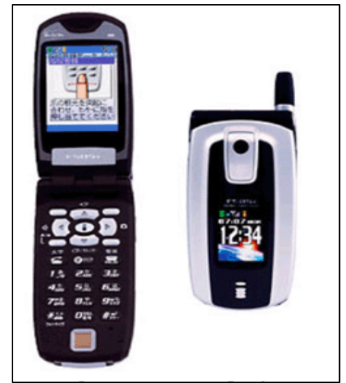
DoCoMo F505i With fingerprint sensor
