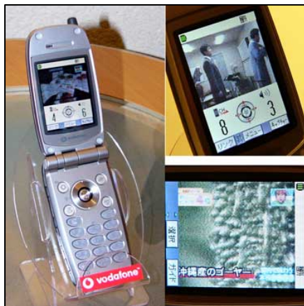
Vodafone V601N With built-in TV tuner
