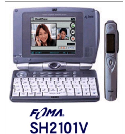
DoCoMo SH2101V PDA-style terminal with detachable pen-sized handset
